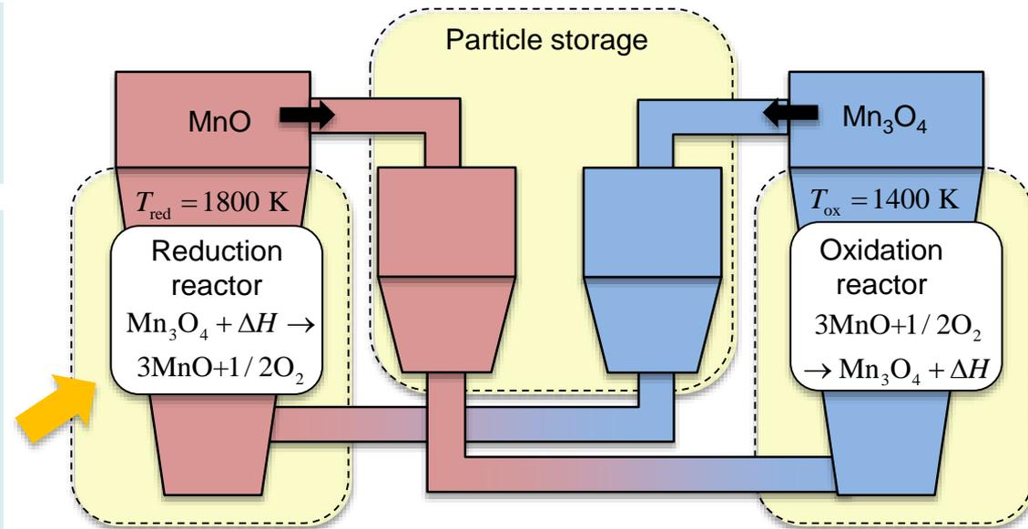
Fig 1. Schematic of a high-temperature solar thermochemical energy storage system for dispatchable and efficient power generation.
