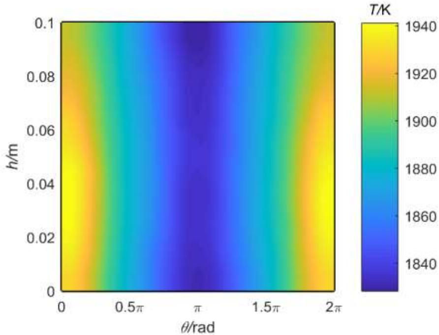
Fig 7. Temperature distribution on the reactor tube outer surface. The azimuthal angle of 0 and  $2\pi$  represent the direction facing the aperture.
