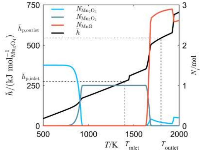
Fig 3. Molar specific enthalpy of the reactive mixture and amount of substance of mixture components.
