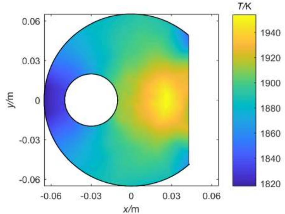
Fig 8. Temperature distribution on the cavity bottom surface.
