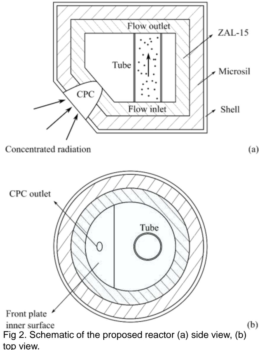
Fig 2. Schematic of the proposed reactor (a) side view, (b) top view.
