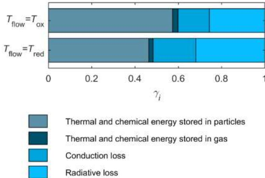
Fig 9. Energy balance of the reactor at steady state with different assumed flow temperatures.
