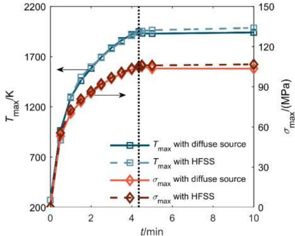
Fig 11. Maximum temperature and thermal stress in the reactor tube with different radiation sources.
