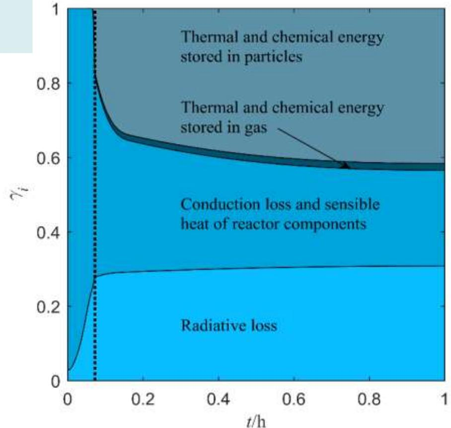
Fig 10. Instantaneous energy balance of the reactor.
