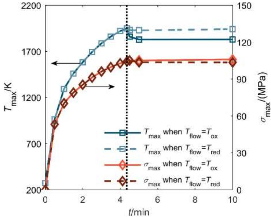
Fig 5. Peak temperature and thermal stress of the reactor tube.
