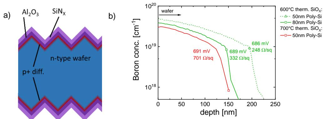
Figure 1 - a) Sketch of the measured symmetrical test structure after the poly-Si is etched off and the surface is re-passivated by Al<sub>2</sub>O<sub>3</sub>/SiN<sub>x</sub>. b) Boron doping profiles measured by ECV for different SiO<sub>x</sub> temperatures and Poly-Si thicknesses. The sheet resistance as well as the iV<sub>OC</sub> values after re-passivation with an Al<sub>2</sub>O<sub>3</sub>/SiN<sub>x</sub> stack are indicated next to each condition.
