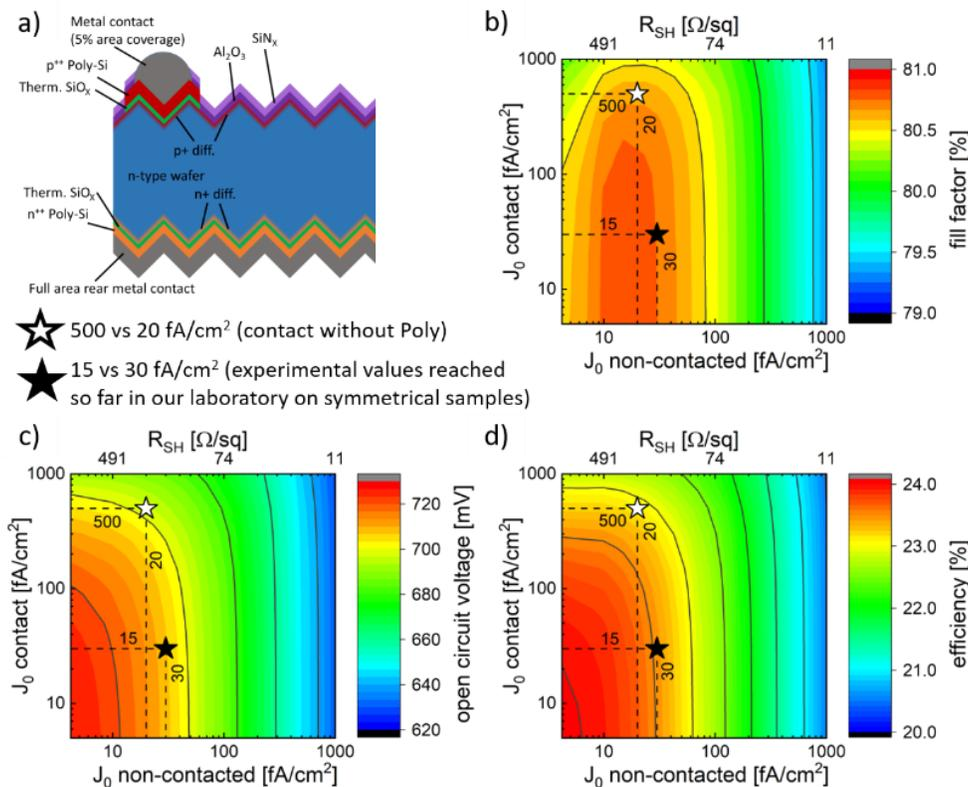
**Figure 2 - a) Solar cell structure used for the simulations. b) fill factor, c) open-circuit voltage and d) efficiency as a function of  $J_0$  below the metallization ( $J_{0,\text{contact}}$ ) versus  $J_0$  between the fingers ( $J_{0,\text{non-contacted}}$ ).**
