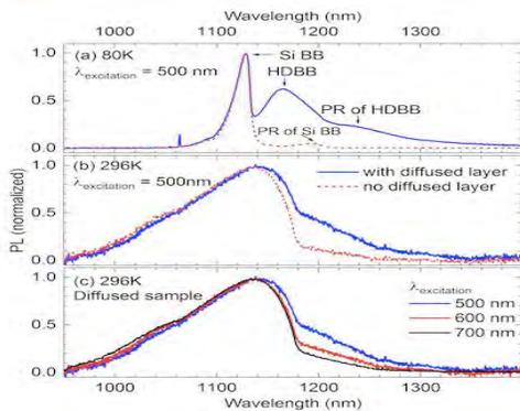
**Fig. 2 (a) (b):** Comparison of normalized PL spectra from c-Si samples with and without a diffused layer captured with the 500-nm excitation wavelength at (a) 80 K (two peaks if there is a diffused layer) and (b) 296 K (only one peak even though the diffused layer exists)
