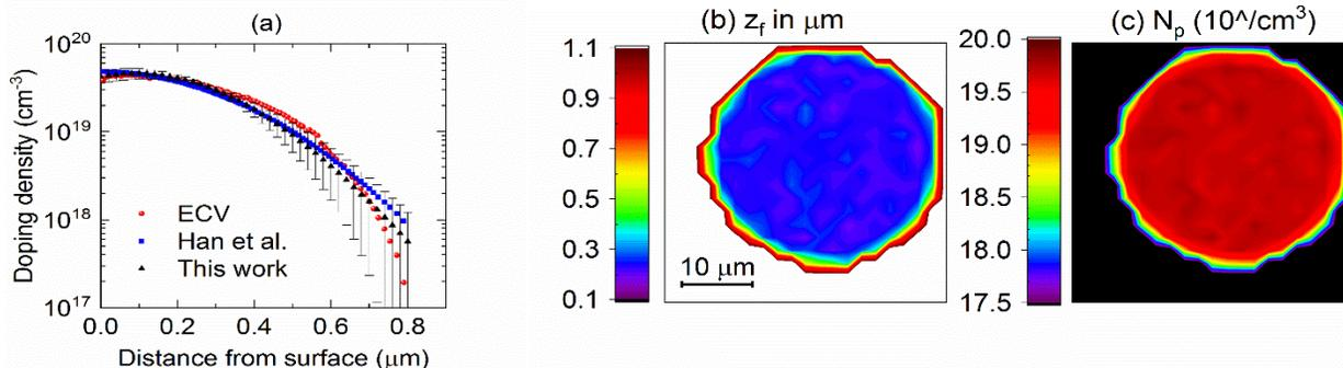
**Fig. 3:** (a) Comparison of dopant profiles among ECV measurements (red circles), Han *et al.*'s method at 80 K<sup>1</sup> (blue squares), and this work at room temperature (black triangles). The error bar is ± one standard deviation, obtained from fifteen data points in the 1 cm × 1 cm diffused area of the patterned wafer. (b)  $z_f$  and (c)  $N_p$  maps of a localized boron-diffused region in the PERL solar cell precursor.
