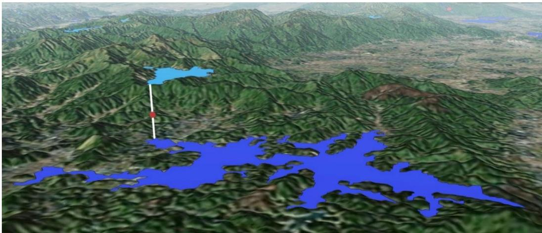
Figure 3. 3D visualisation of a Class-A off-river pumped hydro site in Southern China. Dam heights are adjusted to achieve the water volume required for the target energy storage.
