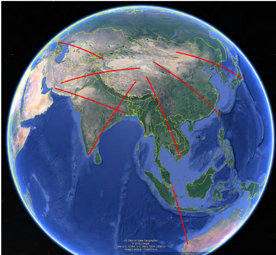
*Figure 1: Asia has excellent solar and wind resources (see maps below). Most of the world's population resides within HVDC-range (3000 km) of central Asia, However, Australia is out of HVDC range of global population centres except for Indonesia. The red bars are each 3000km long. Map: Google Earth.*
