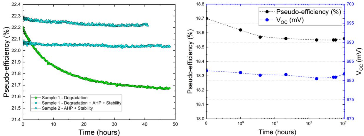
**Figure 1. Left: in-situ monitoring of pseudo-efficiency curves for p-type Cz SHJ cells which underwent 48 hour light soaking LID tests, right: in-situ monitoring of pseudo efficiency and  $V_{OC}$  of p-type mc-Si which has undergone AHP treatment.**
