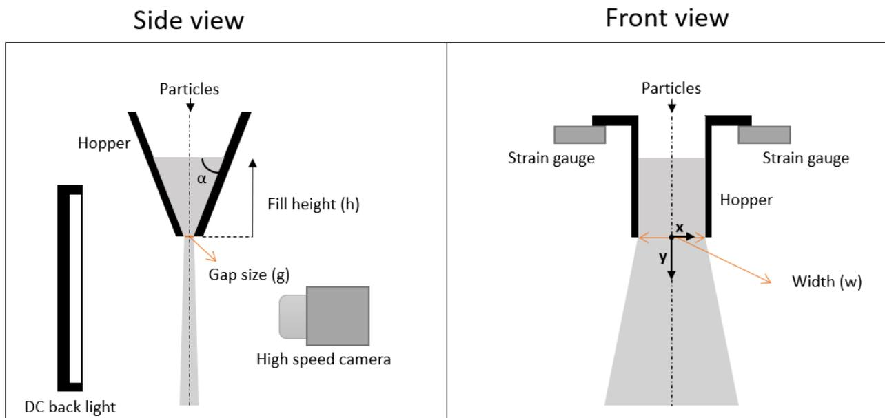
**Figure 1: A schematic of the side and front view of the experimental setup**
