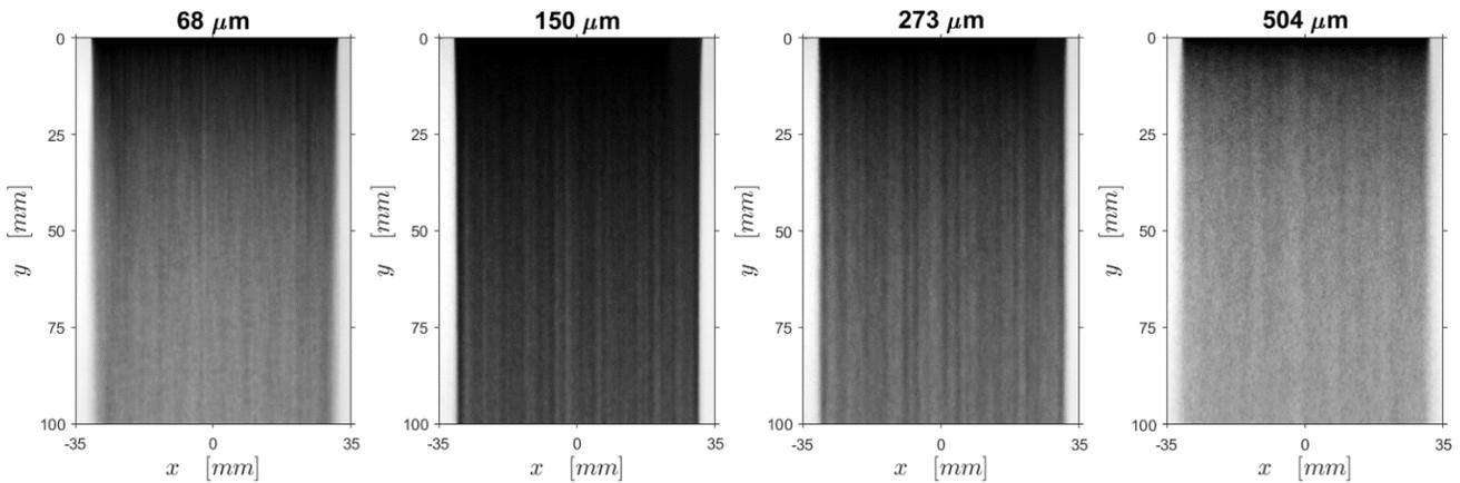
**Figure 2. Time averaged images from the front of the particle curtain for 4 different particle sizes. The particle flow is from top to bottom.**
