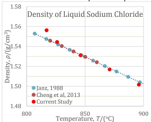
**Figure 2. Theoretical (Janz, 1988) and experimental (Cheng et al, 2013 and current study) comparisons of liquid density for the single component salt, sodium chloride.**
