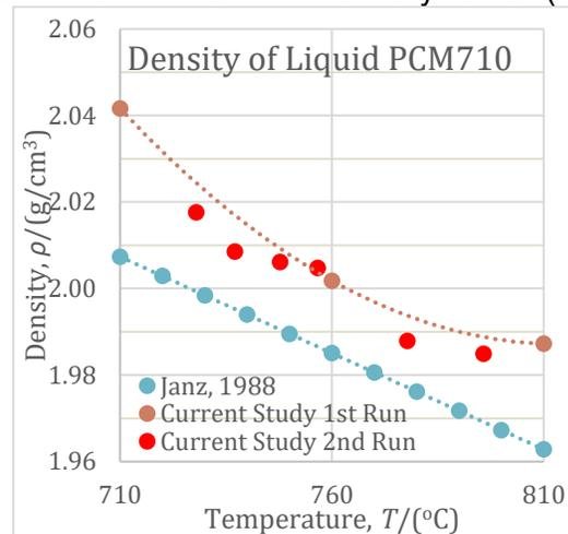
**Figure 3. Comparison between theoretical (Janz, 1988) and experimental (current study) liquid density of the multi-component salt, PCM710.**
