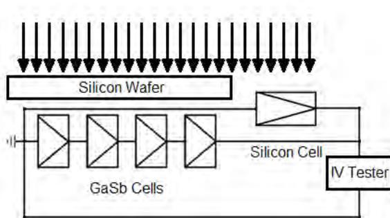
Figure 3. Schematic for the intermediate-band solar cell analogue circuit.
