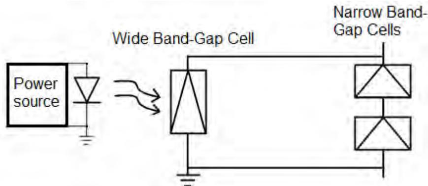
Figure 5. Potential schematic for multiple-exciton generation analogue.
