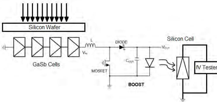
Figure 1. Schematic for the up-conversion circuit.
