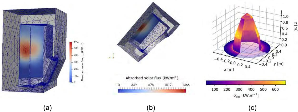
**Fig 1. Sodium receiver design options showing absorbed flux for three different concepts: (a) Abengoa/CSIRO CO<sub>2</sub> receiver selected for initial testing; and two higher-performance concepts from (b) CSIRO and (c) ANU under consideration for the second phase of testing.**
