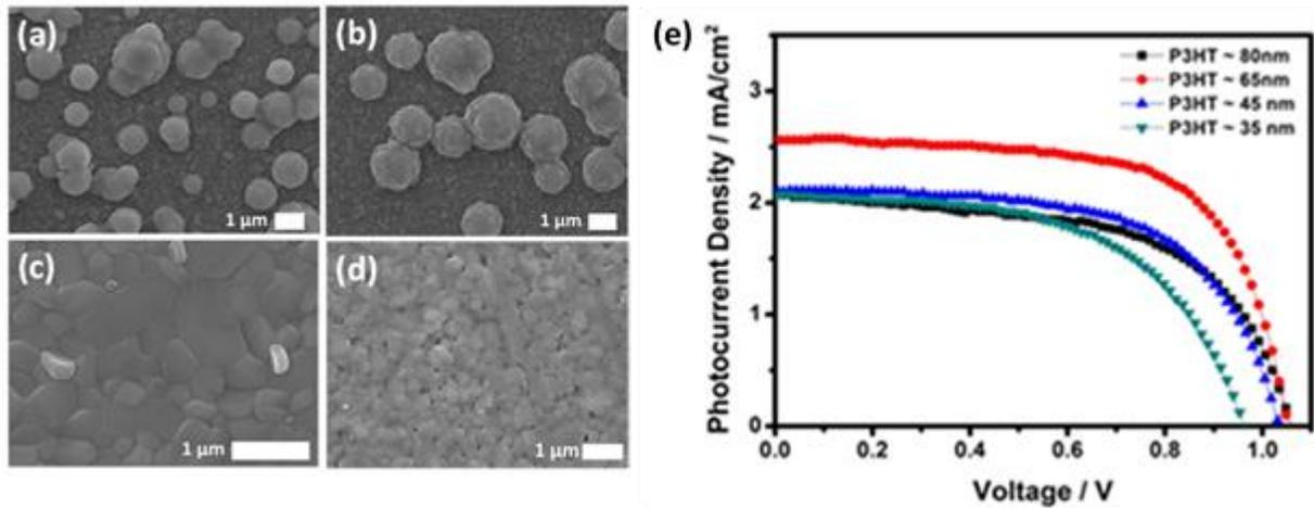
**Figure 3. Scanning electron microscope (SEM) images of Cs<sub>2</sub>AgBiBr<sub>6</sub> on FTO at different spin coating rate (a) 2000 rpm, (b) 3000 rpm, (c) 4000 rpm, (d) 5000 rpm. (e) J-V curve of devices based on planar structure of FTO / C-TiO<sub>2</sub> / Cs<sub>2</sub>AgBiBr<sub>6</sub> / P3HT / Cu under 1 SUN illumination with different P3HT thickness**
