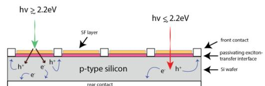
**Figure 3. Schematic of a potential singlet fission enhanced front-contact c-Si solar cell.**
