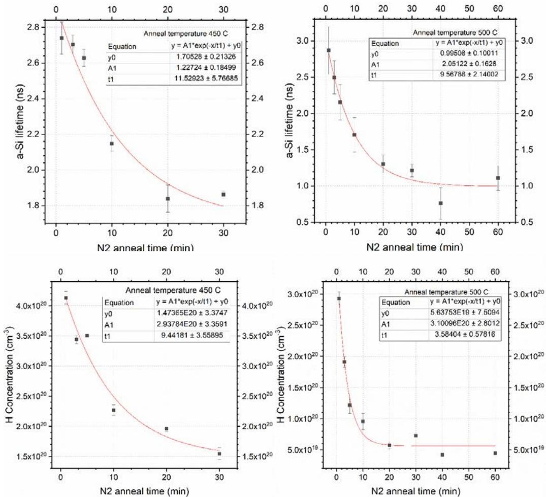
**Figure 1 Comparison of the effective lifetime, a-Si lifetime as well as the hydrogen concentration of the samples when annealed at temperature 450 °C (left column) and 500 °C (right column).**
