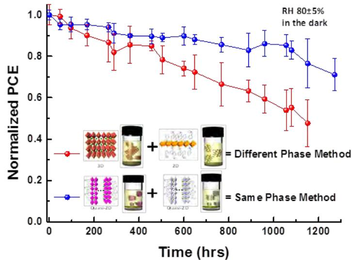
**Figure 1 Normalized PCE of DP and SP un-encapsulated solar cells during exposure to RH 80±5% in the dark. Cells using different perovskite precursor preparations show different stabilities**
