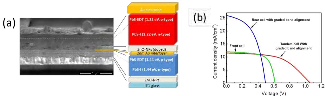
Figure 1 (a) Illustration of the structure of tandem PbS CQD solar cells. (b) J-V curves of fabricated tandem cell and single-junction cells with graded band alignment.
