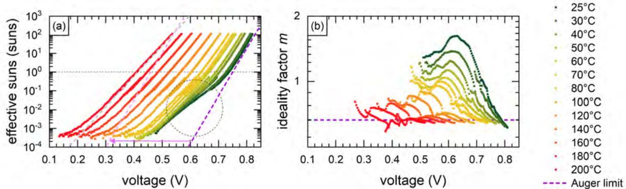
**Figure 2 (a) Temperature-dependent Suns- $V_{oc}$  data with different slopes indicated by dashed lines. (b) Voltage-dependent ideality factor  $m$  calculated from Figure (a). Note that the data has been cropped and  $m$  calculated averaging over 13 points.**
