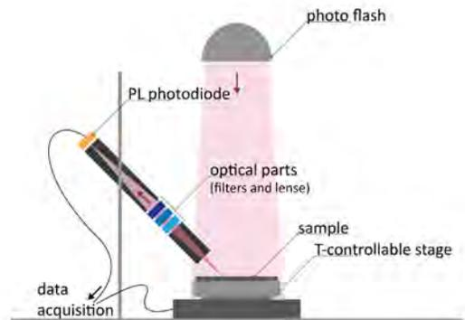
**Figure 1 Simplified sketch of the setup used in this study. The arrows indicate the path of the light or signals.**
