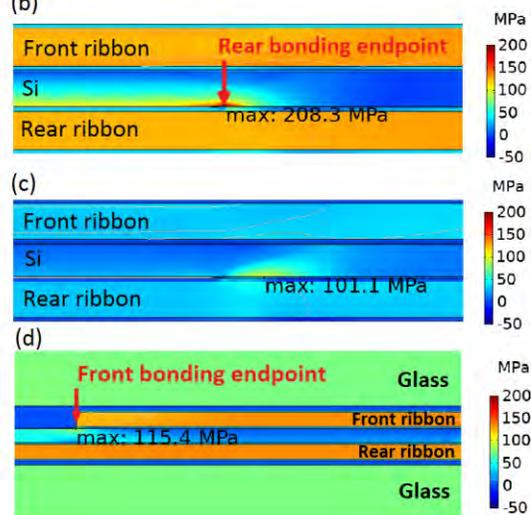
Figure 1(c)]. During the initial lamination cooling from 150 °C to 110 °C, the maximum tensile stress decreases as the glass compression counteracts the solder-induced tensile stress. Within this temperature range, the maximum stress remains at the rear bonding endpoint. With further decrease in temperature, the maximum tensile stress starts to increase, which is attributed to the transition of
