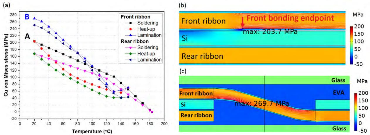
**Figure 2. (a) Simulated von mises stress in Cu ribbons after soldering, heat-up and lamination; (b) stress mapping at 20 °C after soldering (point A on graph(a)); and (c) stress mapping at 20 °C after lamination (point B on graph(a)).**
