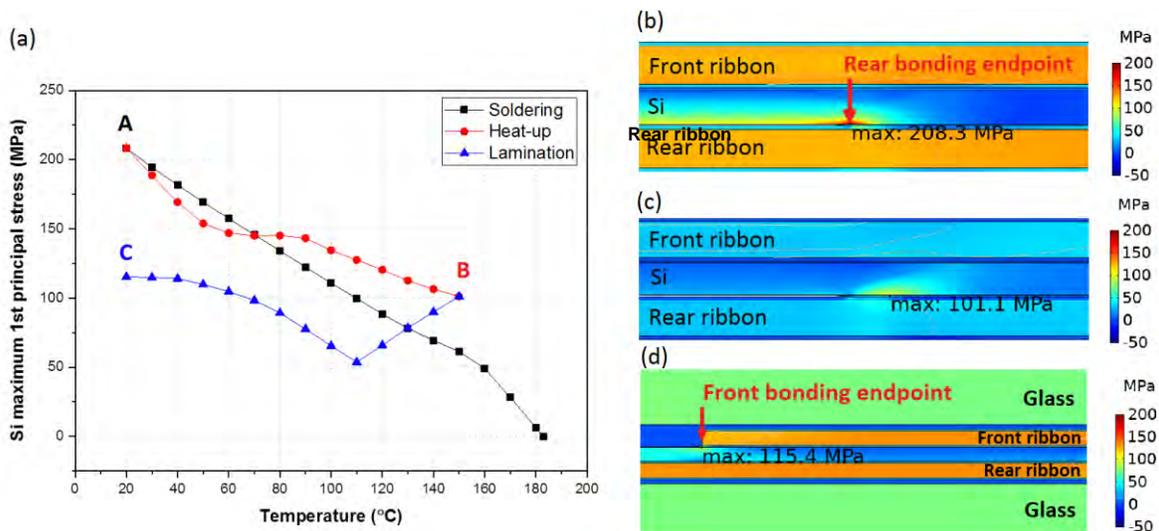
**Figure 1. (a) Simulated 1st principal (tensile) stress in Si after soldering (black), heat-up (red) and lamination (blue); (b) stress mapping at 20 °C after soldering (point A on graph(a)); (c) stress mapping at 150 °C after heat-up (point B on graph(a)); and (d) stress mapping at 20 °C after lamination (point C on graph(a)).**
