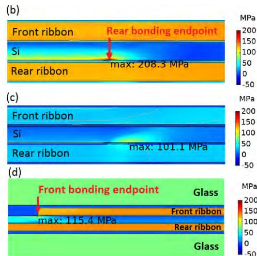
Figure 1(a) shows the evolution of 1<sup>st</sup> principal (tensile) stress in Si undergone soldering (black curve), laminate heat-up (red curve) and glass-glass module lamination (blue curve). During soldering the Si tensile stress increases approximately linear with decreased temperature. At 20 °C the maximum stress is 208 MPa located at the rear bonding endpoint [see
