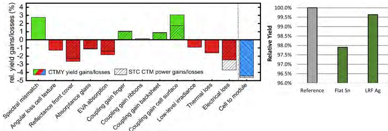
**Figure 2. (left) Relative annual yield gains and losses for a 72-cell monocrystalline PERC module under realistic conditions in Melbourne. (right) Relative yield for the same module with flat Sn ribbons and LRF ribbons normalized to the ideal reference.**
