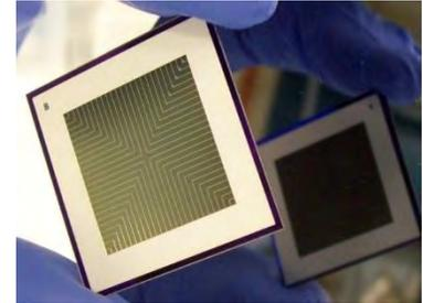
*Figure 3: Completed bifacial solar cell fabricated for this work.*
