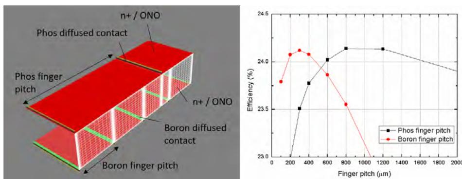
Figure 2: (Left) 3D mesh of bifacial unit-cell simulation, and (Right) the 3D simulation results to deduce optimum n-finger and p-finger pitch.
