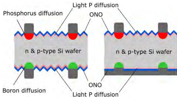
Figure 1: Cross-sectional view of bifacial and mono-facial cell design in this work
