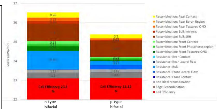
*Figure 4: (Left) Optical loss breakdown, (Right) Free-Energy-Loss-Analysis comparison between n-type and p-type bifacial solar cells.*
