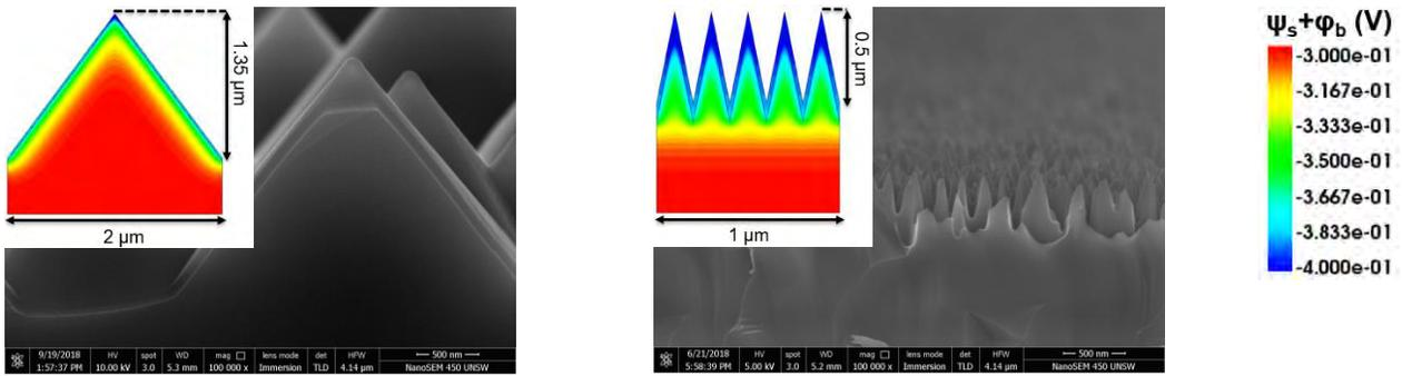
Figure 1. The 2D models of random pyramid and b-Si according to the SEM images of the real surface texturing. The models also show the surface band bending at high  $Q_f$ .
