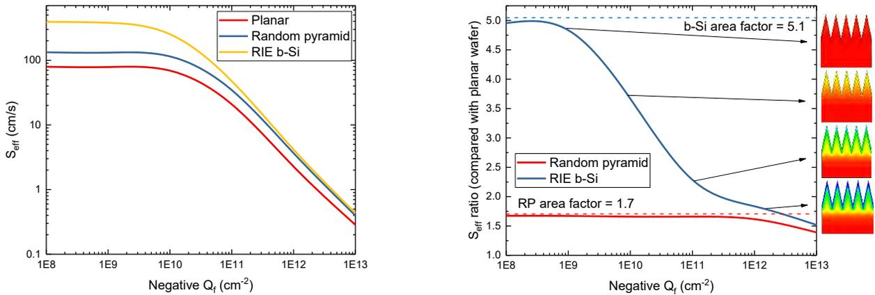
Figure 2. (a) Simulated  $S_{\text{eff}}$  against  $Q_f$  for planar, random pyramid and b-Si, and (b)  $S_{\text{eff}}$  ratio based on the planar surface for random pyramid and b-Si with different  $Q_f$ . The band bending conditions of b-Si are also shown when  $Q_f = 10^9, 10^{10}, 10^{11}$  and  $10^{12} \text{ cm}^{-2}$ .
