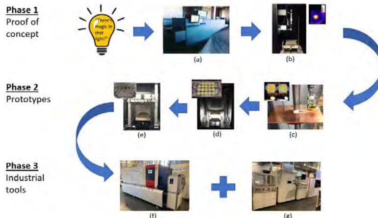
Figure 1. Toolset in various developmental stages of the AHT. (a) Schmidt belt-furnace; (b) laser prototype for small samples; (c) LED prototype for small samples; (d) LED prototype for 6" samples; (e) final LED prototype for 6" samples; (f) ANT tool; (g) DR Laser tool.
