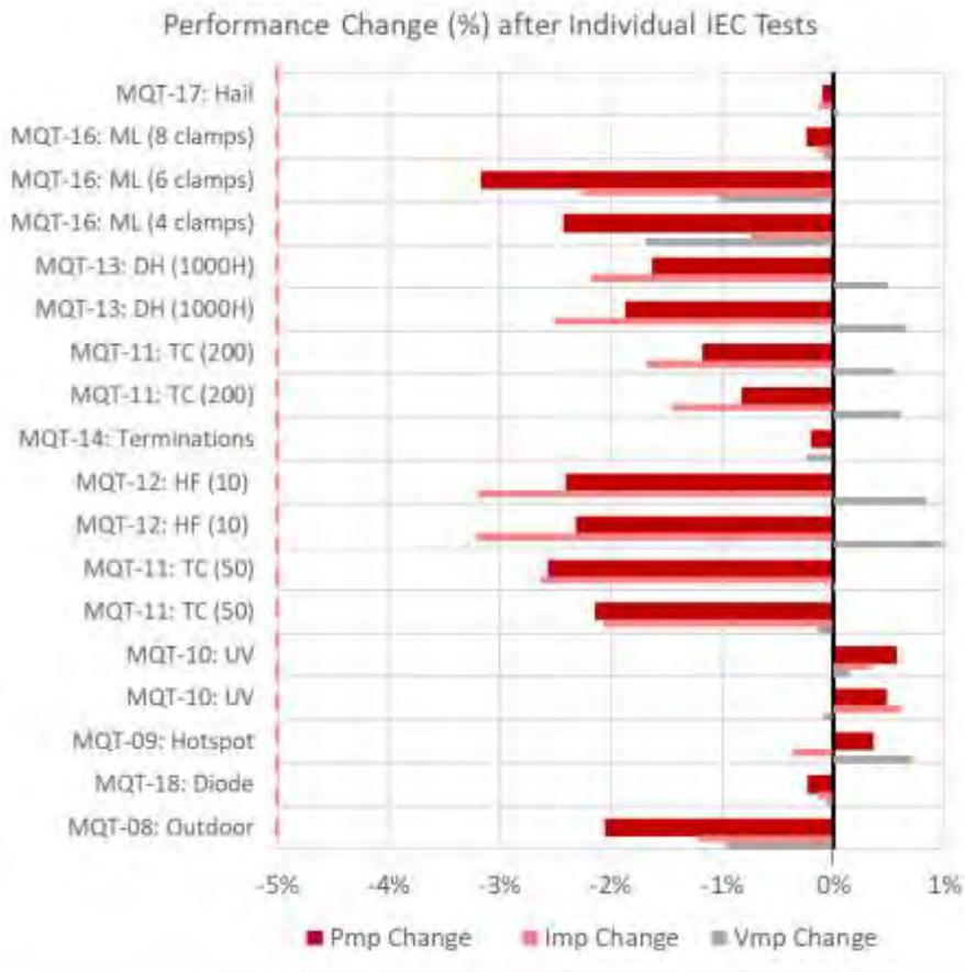
**Figure 1. Performance change in IEC testing, compared to the performance degradation threshold. See [2] for further information on individual tests. Note that some tests, such as MQT-11:TC (50) are done in a sequence after other tests.**
