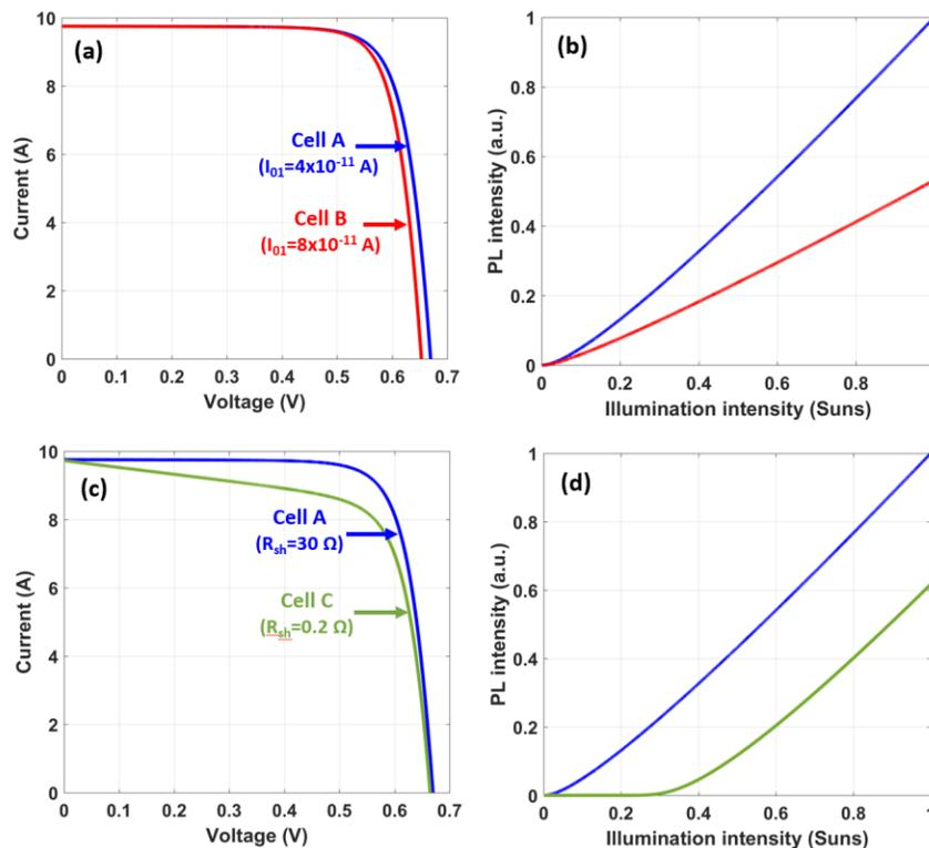
**Figure 1. Comparison of the I-V curve of a typical cell (Cell A) with simulated I-V curve of a cell with increased (a) base recombination current (Cell B) and (c) shunt resistance (Cell C) along with the cells' PL (b and d) as a function of illumination.**
