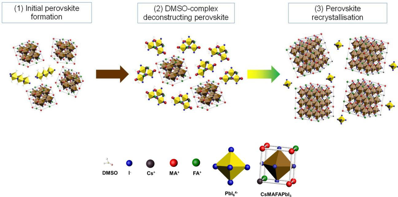
**Figure 2** Schematic showing phase transition during the second step of sequential processing: (a) Phase 1 - initial perovskite formation; (b) Phase 2 - perovskite deconstruction due to the formation of (MA/FA/Cs)<sub>4</sub>PbI<sub>6</sub>-2DMSO complex); (c) Phase 3 - perovskite re-crystallisation.
