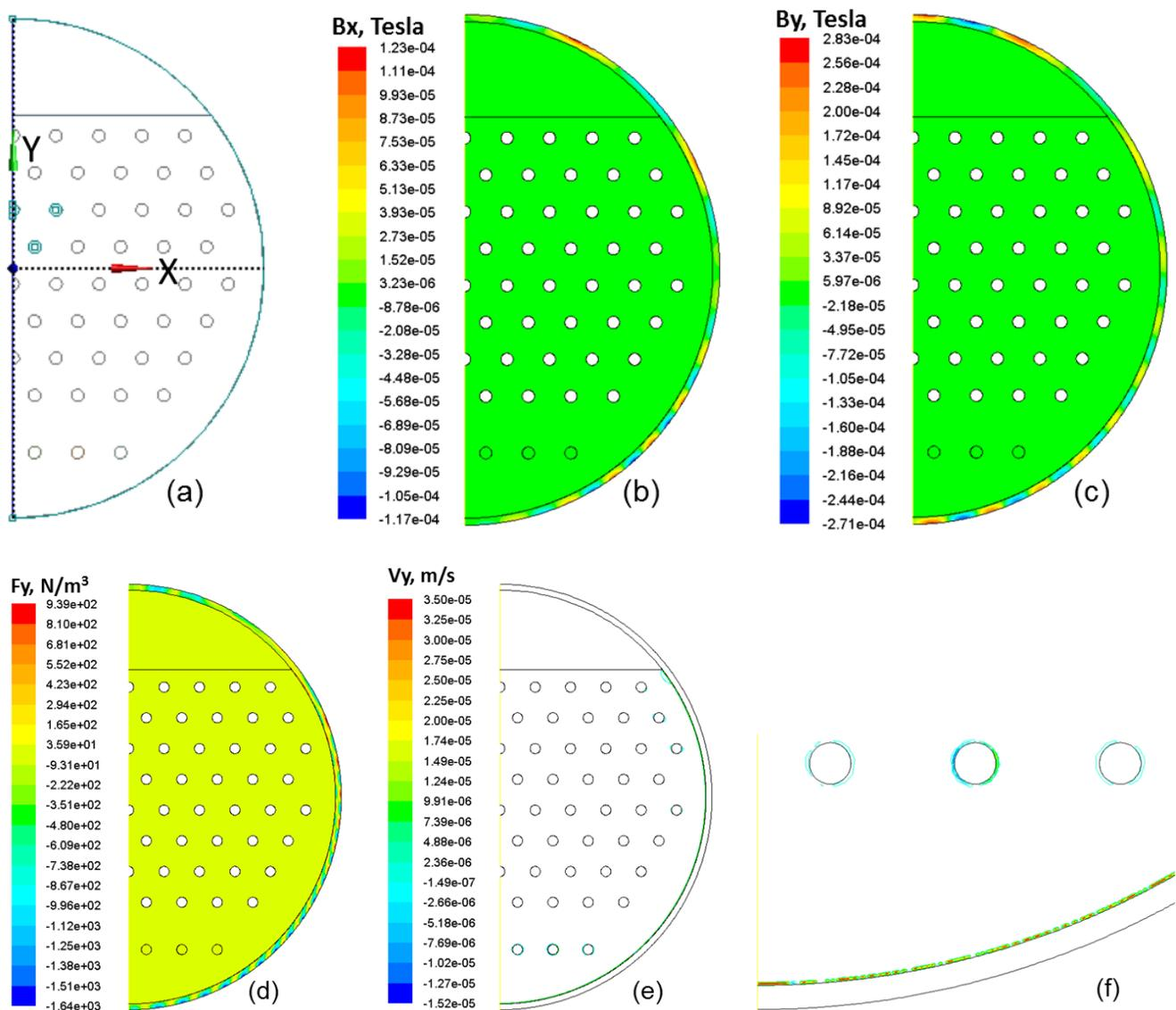
**Figure1-** (a) Schematic of the grid, (b) Induced Magnetic field in X direction, and (c) in Y direction, (d) Induced Lorentz force in Y direction, (e) Velocity in melted PCM in Y direction, (f) Zoom view of  $V_y$  showing eddy current in melt region close to shell and electrical heater surfaces
