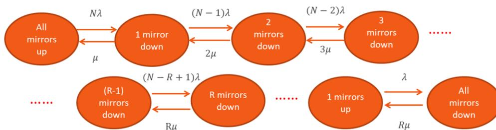
**Figure 1. Markov process for failure and repair of mirror field**
