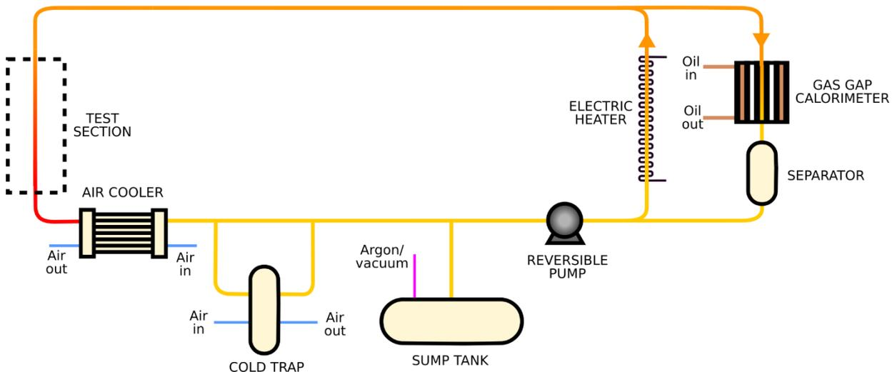
**Figure 1. Process flow diagram for ANU sodium laboratory**
