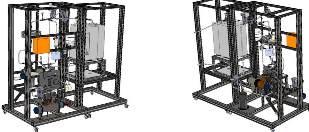
**Figure 2. Assembly drawing of the ANU sodium laboratory from front (left) and back (right)**
