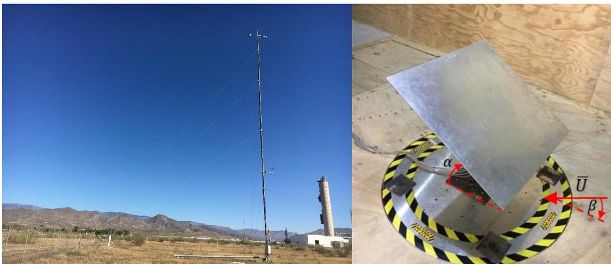
**Figure 1. Meteorological mast at the PSA heliostat field site (left); model-scale heliostat load measurements in the University of Adelaide wind tunnel (right).**
