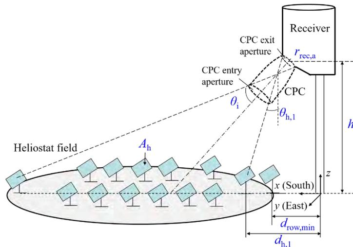
**Figure 1. A model solar central receiver optical system with a heliostat field, a central tower, a receiver and an optional CPC.**
