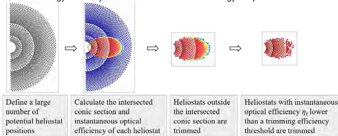
**Figure 2. Determination of heliostat field boundary as implemented in this study [12].**
