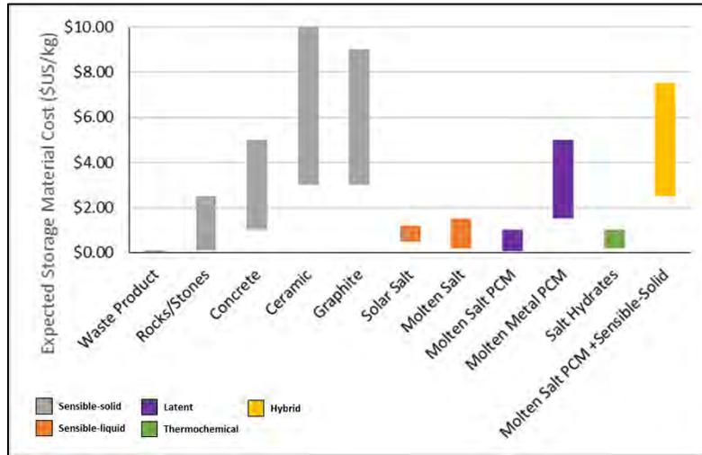
**Figure 2- Expected Storage Material Cost for Several TES Concepts**
