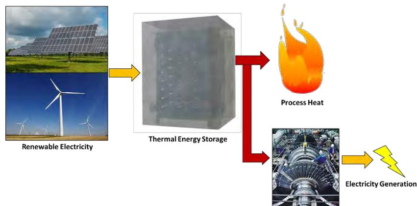
**Figure 1- Basic Schematic of a Thermal Battery**
