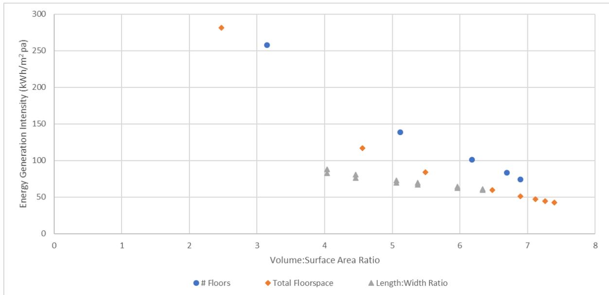
**Figure 5. Generation Potential vs Compactness Factor (Volume: Surface Area)**
