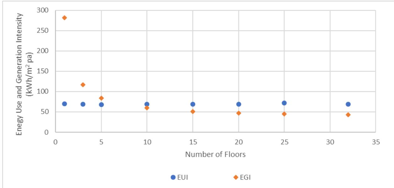
**Figure 3. Energy Use Intensity/Energy Generation Intensity vs Total Floorspace**
