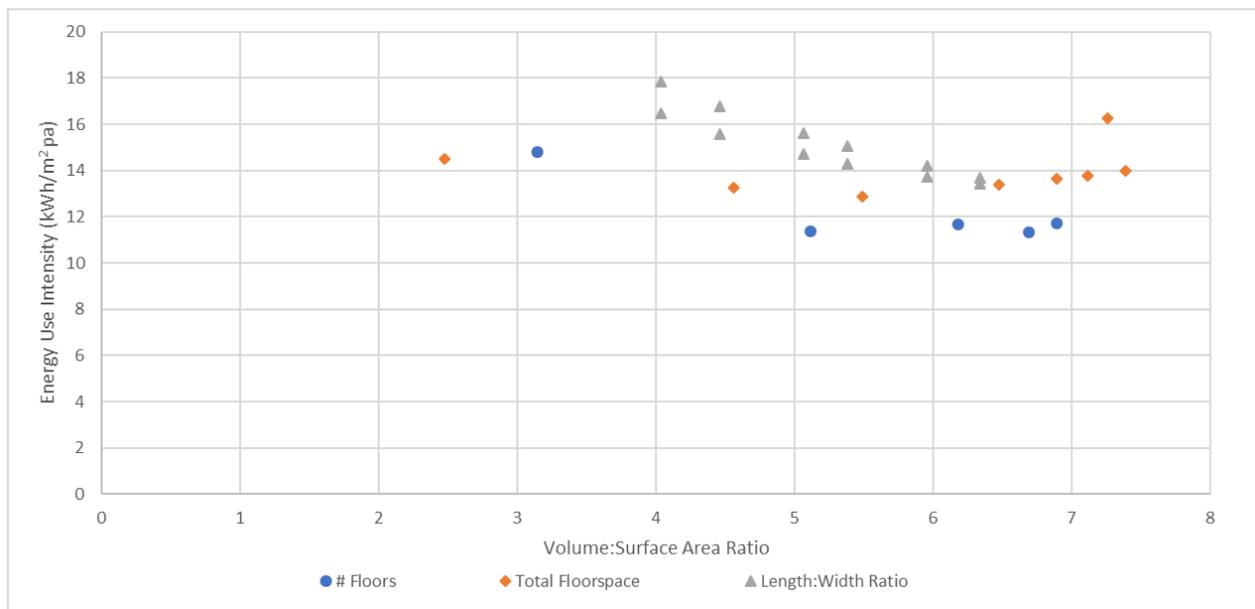
**Figure 4. HVAC Energy Use Intensity vs Compactness Factor (Volume: Surface Area)**
