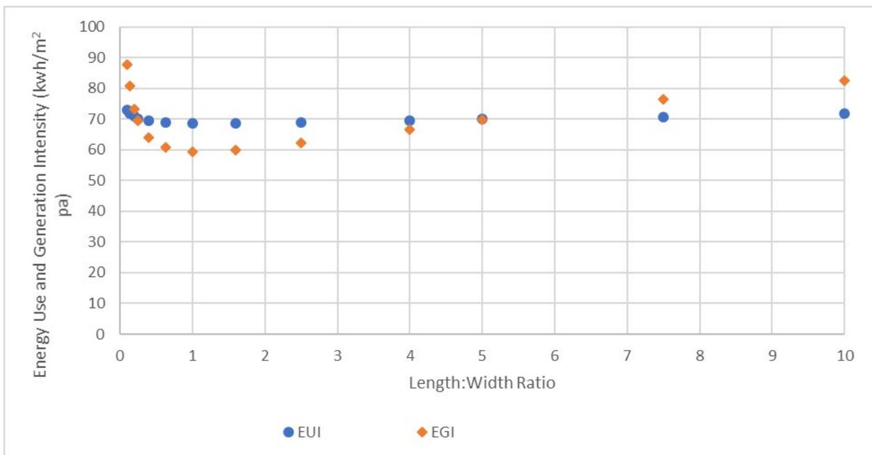
**Figure 2. Energy Use Intensity/Energy Generation Intensity vs Length: Width Ratio**
