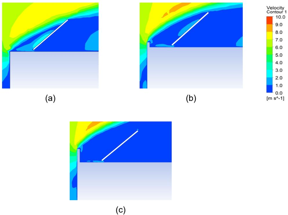
**Figure 6: Flow over a collector at 40° inclination for a) no parapet b) 0.4m parapet and c) 1.2m parapet**
