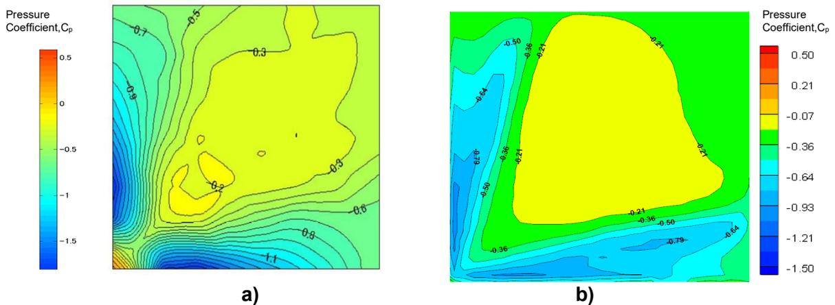
**Figure 2: Mean wind pressure coefficients contour for a 45° wind direction: (a) the TPU aerodynamic database and (b) Results of the present CFD model**
