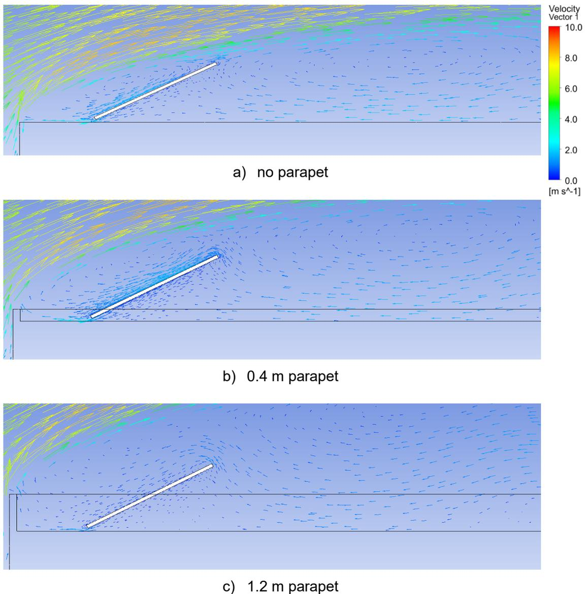
**Figure 4: Velocity vectors for varying parapet heights**
