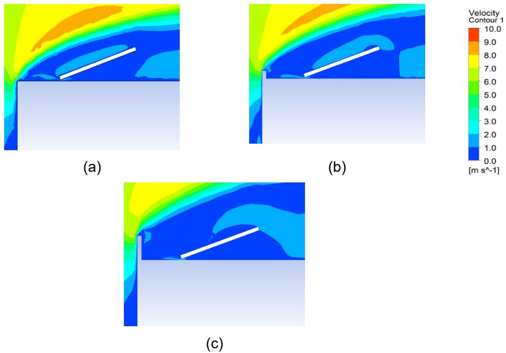
**Figure 5: Flow over a collector at 20° inclination for a) no parapet b) 0.4m parapet and c) 1.2m parapet**
