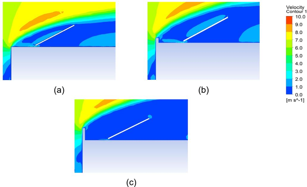
**Figure 3: Velocity contours for a) no parapet b) 0.4m parapet and c) 1.2m parapet**
