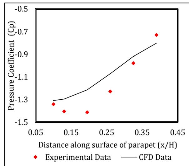
**Figure 1.0:** Comparison of experimental and numerical data for low parapet ( $h/(H+h) \leq 0.09$ ) at 5m/s.
