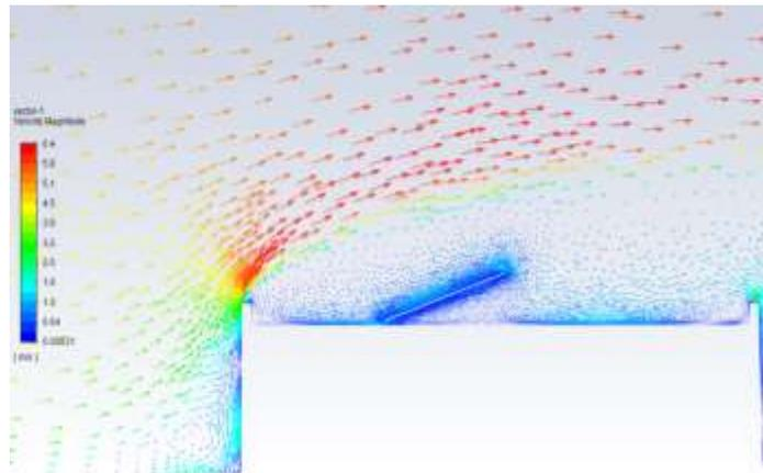
**Figure 2.0:** Flow visualisation around roof mounted collector with perimetric parapet.
