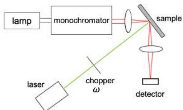
Figure. 3 The basic PR setup
