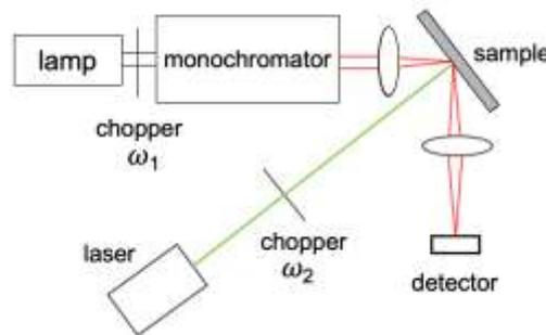
**Figure 4. The double demodulation [7] PR setup.**
