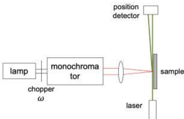
Figure. 2 The basic PDS setup
