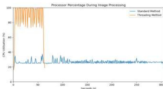
**Figure 1. Processing percentage of the CPU during the image mapping step using the standard loop method and using the multithreading loop method. Note that the process was shortened from 256 image scans to 16 to show more detail.**
