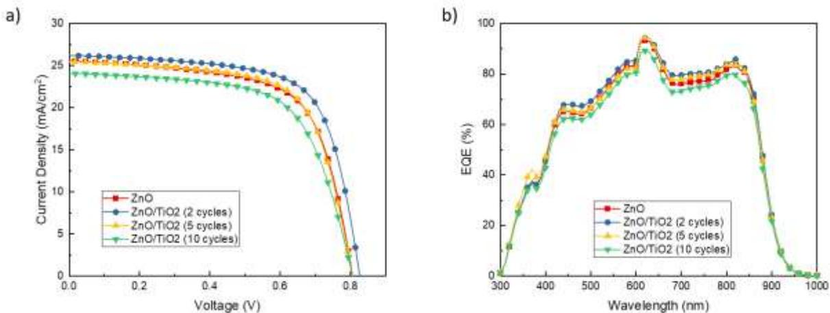
Figure 1. a) Current density to voltage (J-V) curves and b) external quantum efficiency (EQE) spectrum of fabricated OSCs with different ALD cycles of ultrathin TiO<sub>2</sub> layer.
