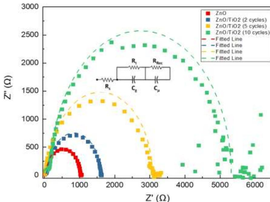
**Figure 2. Nyquist plots with the equivalent electrical circuit at a bias of 700 mV under the dark condition for fabricated OSCs with different ALD cycles of ultrathin TiO<sub>2</sub> layer.**
