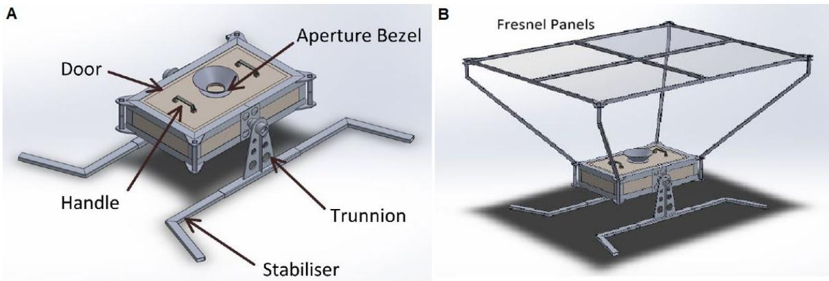
Figure 1 - Schematic of a solar thermal sintering apparatus for producing bricks from lunar regolith. Figure by Minogue et al. [2].
