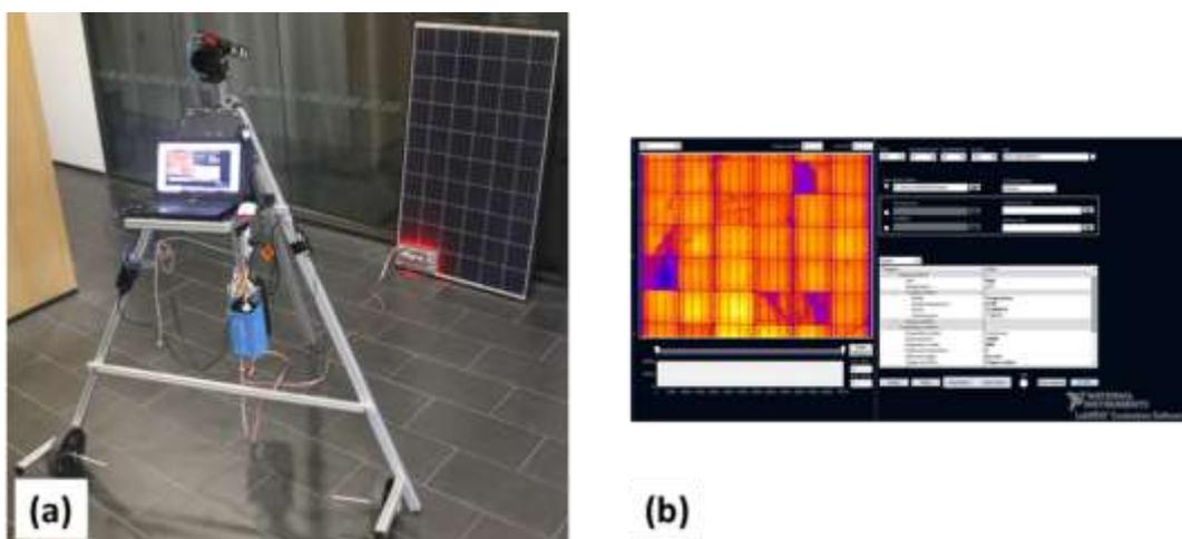
**Figure 2. (a) Alpha prototype outdoor PL tool; (b) screenshot of software used to capture and analyse the images and control the optical modulator.**
