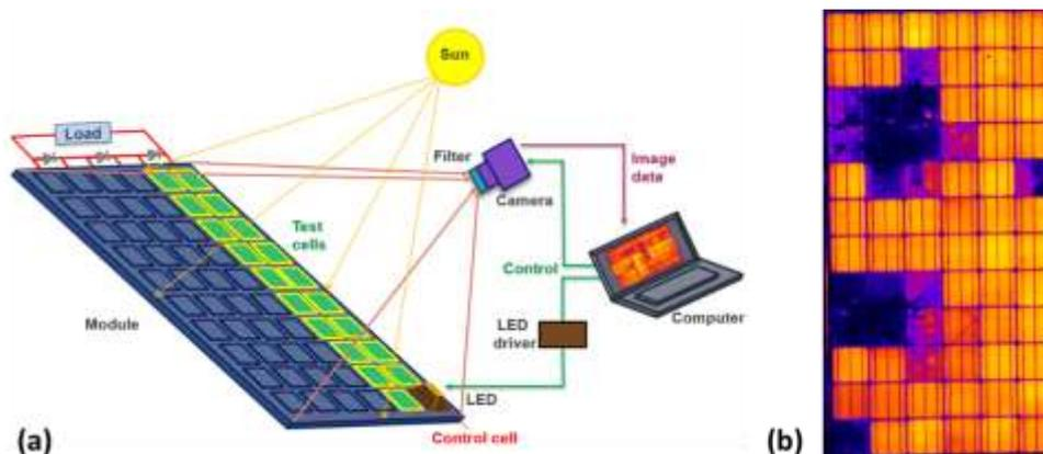
**Figure 1. (a) Schematic of outdoor PL system utilising optical modulation via a high-power LED array; (b) outdoor PL image of a 72 cell silicon PV module.**
