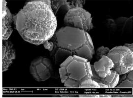
**Figure 2. SEM image of the condensed substance shown the average particle size is less than 3 microns.**
