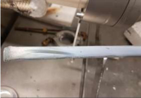
**Figure 1. Condensed substance has whitish appearance near hot zone and greyish appearance closer to the end.**
