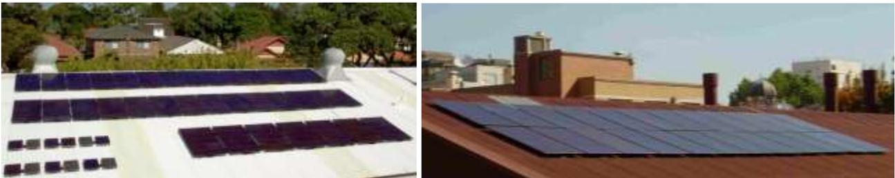
Figure 2. Early field prototypes for lifetime testing, Pilot Line Roof (Left), Power House Museum, Sydney (Right), 2007.
