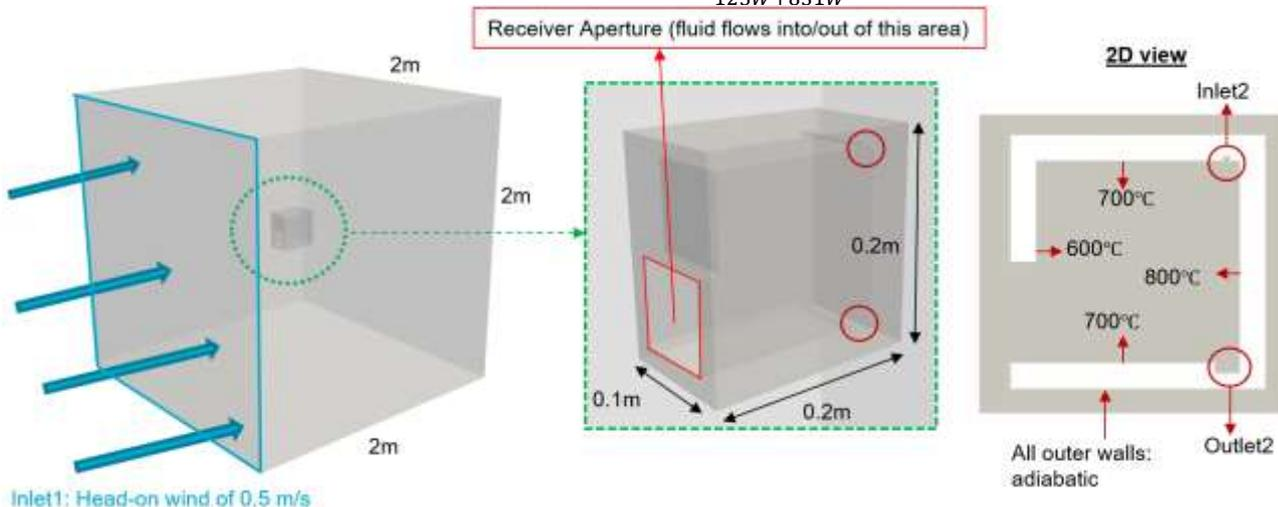
Figure 1. Computational domain of cavity receiver.
