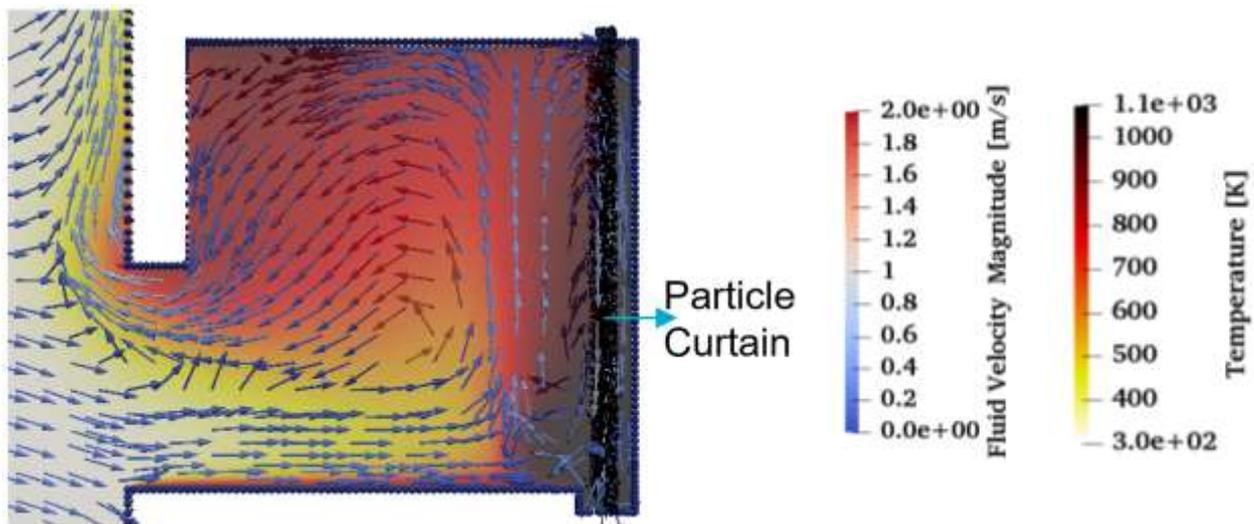
**Figure 2. Close-up view of buoyant convection of solid-gas flows taken at 60 s. Note that the particle curtain is denoted by the dotted region.**
