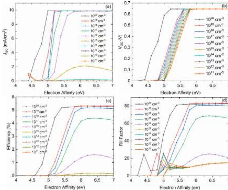
Figure 4. Effect of the trap density in MoO<sub>x</sub> layer on the GaP/Si/a-Si/MoO<sub>x</sub> device performance on (a) short-circuit current, (b) open-circuit voltage, (c) efficiency, (d) fill factor.
