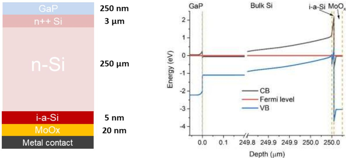
Figure 3. Left: Schematic of Sentaurus simulated GaP/Si/a-Si/MoO<sub>x</sub> structure. Right: Calculated band alignment of the simulated GaP/Si/a-Si/MoO<sub>x</sub> structure.
