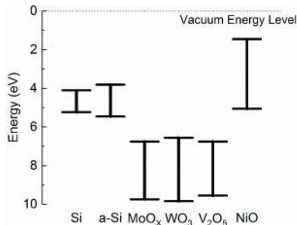
Figure 1. Bandgap and band alignment of some hole selective materials with silicon [3-6].
