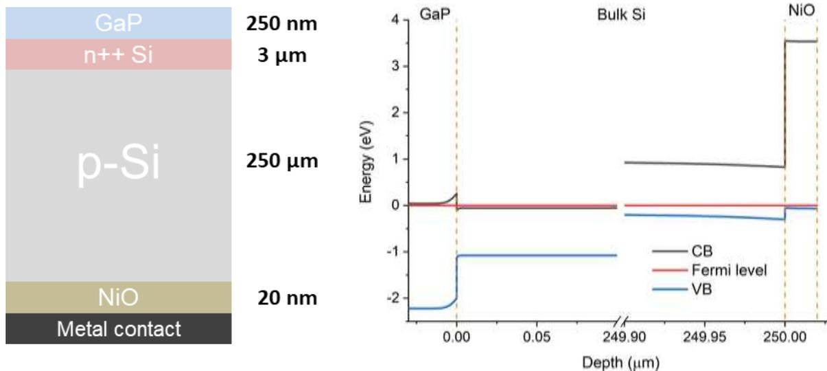
Figure 2. Left: Schematic of Sentaurus simulated GaP/Si/NiO structure. Right: Calculated band alignment of the simulated GaP/Si/NiO structure.
