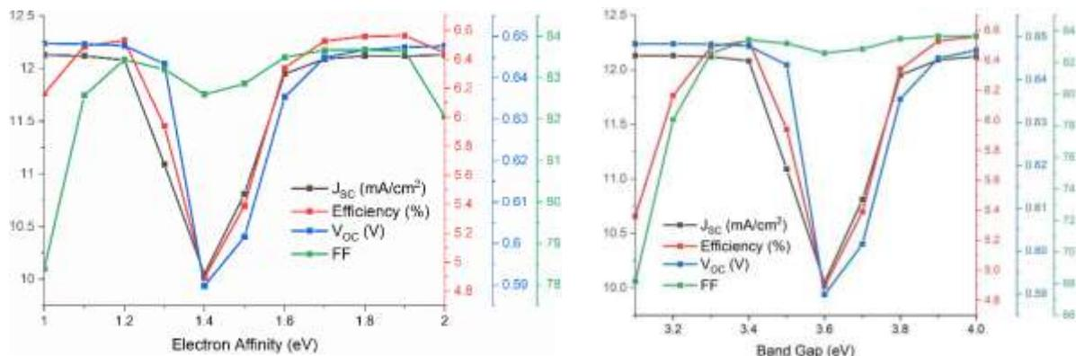
Figure 3. Simulated effect of Left: electron affinity, Right: Bandgap value of NiO on the cell performance.
