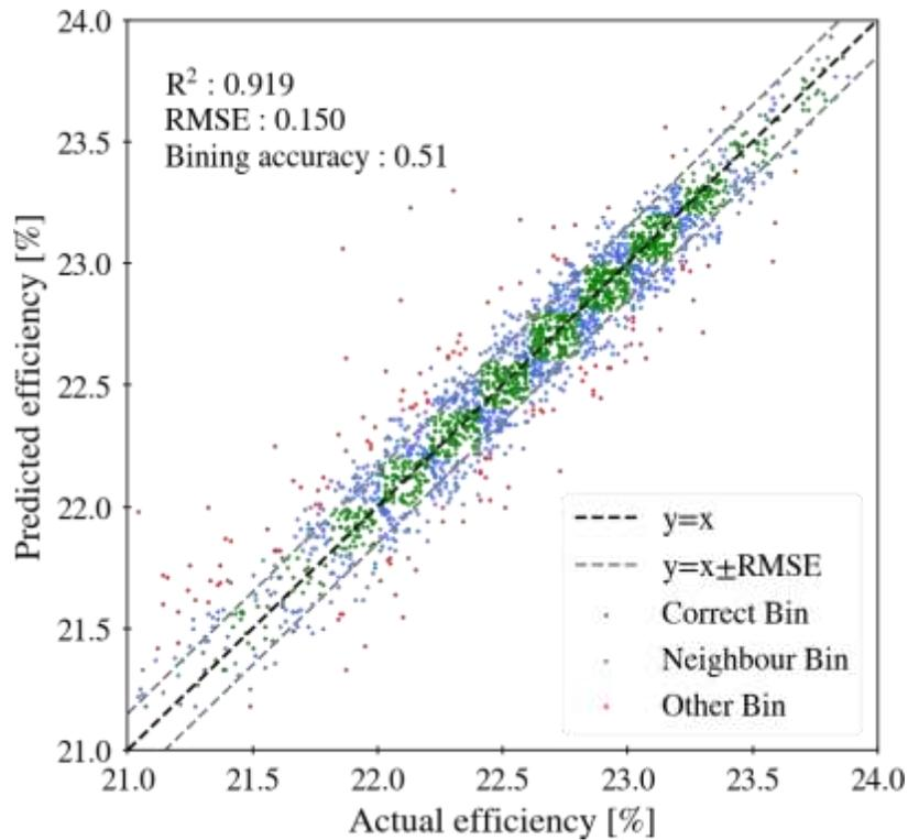
**Figure 1. True vs predicted efficiency for validation set Val<sub>2</sub> using the best performing AdaBoost model after EL-Net feature extraction.**
