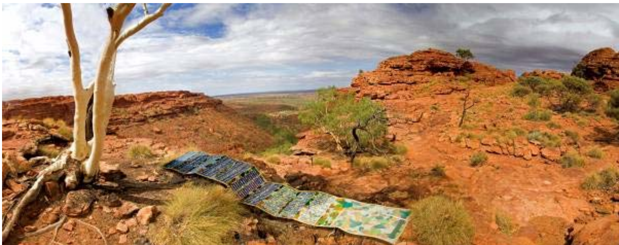
Figure 10: DSC modules are under test for the Australian defence force. Photo: Dyesol
