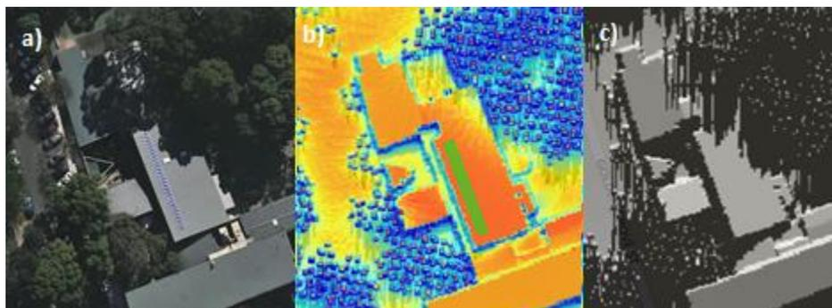
**Figure 1: a) Aerial image of Darlington PS PV System; b) Insolation heat map kWh/m<sup>2</sup>/day; c) Winter solstice midday shadows.**
