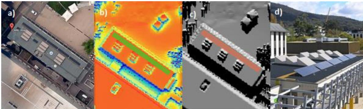
**Figure 3: a) Aerial image of ANU Building 17 PV System; b) Insolation heat map kWh/m<sup>2</sup>/day; c) Winter solstice midday shadows; d) Image of ANU building 17 PV systems as portrayed on SMA's Sunny Portal**
