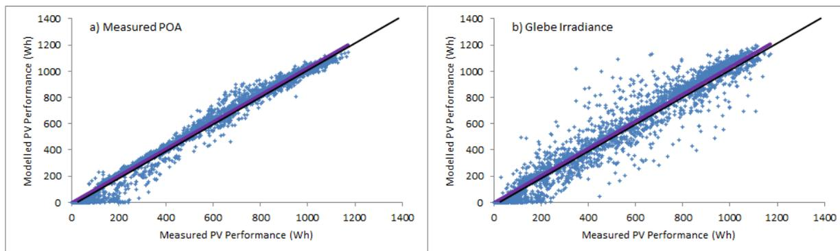
**Figure 5: Measured vs. modelled AC power for a PV system located in Alexandria using a) onsite measured POA and b) POA irradiance measured in Glebe**
