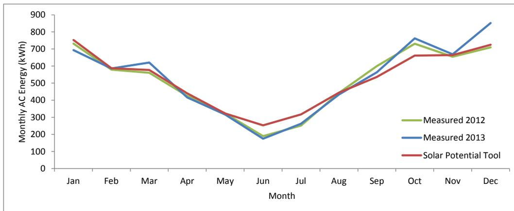
**Figure 2: Monthly AC output in kWh measured for the years 2012 and 2013 in comparison to the APVI Solar Potential Tool**
