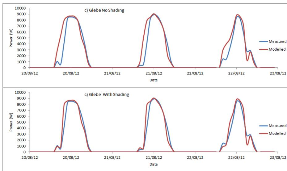
**Figure 7: Measured vs. modelled AC power with and without shading modelled**
