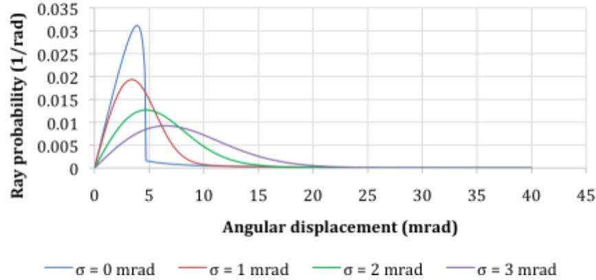
**Figure 3: Directional probability distribution of reflected rays for a range of mirror slope and tracking errors ( $\sigma$ ).**
