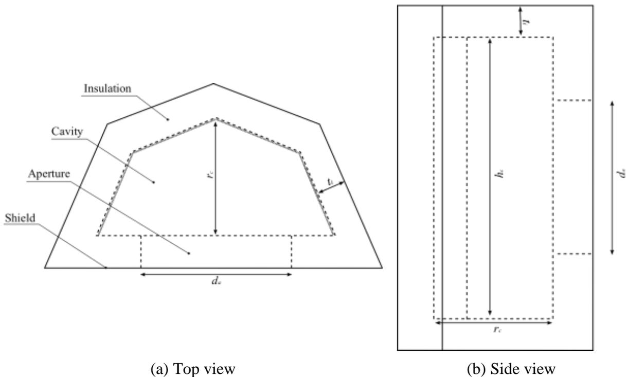
**Figure 1: Illustration of cavity receiver geometry.**
