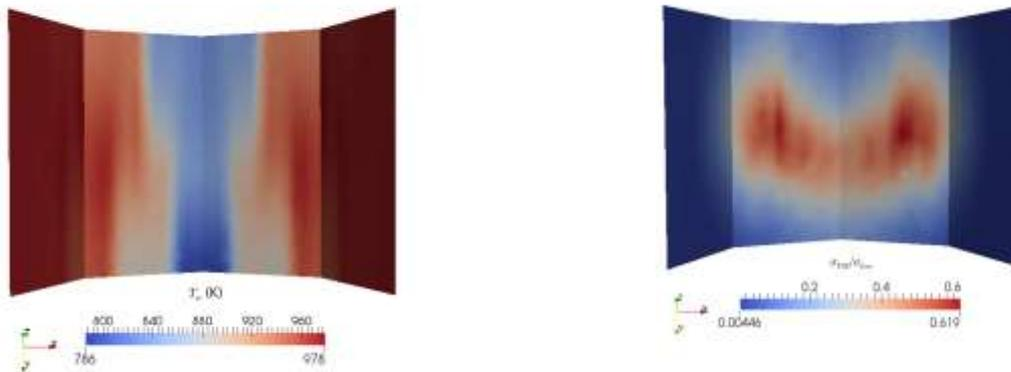
(a) Surface temperature on the receiver panels.
