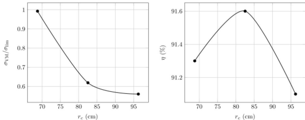
(a) Ratio of von Mises stress to ASME boiler code strength limit.
