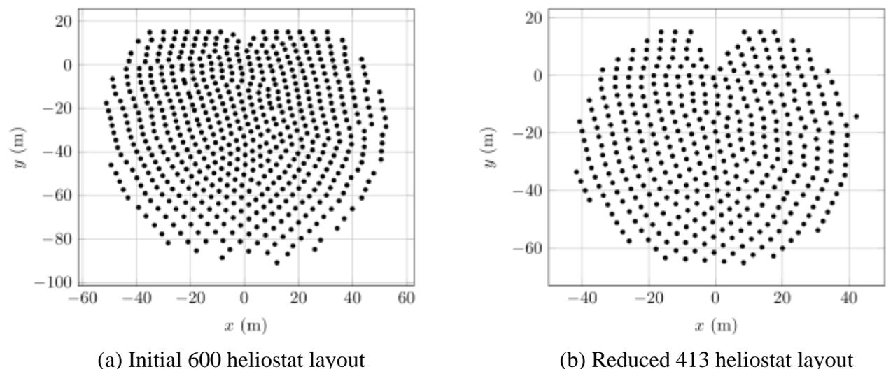
**Figure 7: Optimised heliostat layout for best aperture setup ( $r=55$  cm,  $\theta=60^\circ$ ,  $h=30$  m).**
