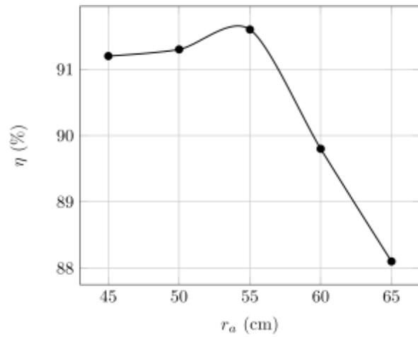
(b) Receiver thermal efficiency
