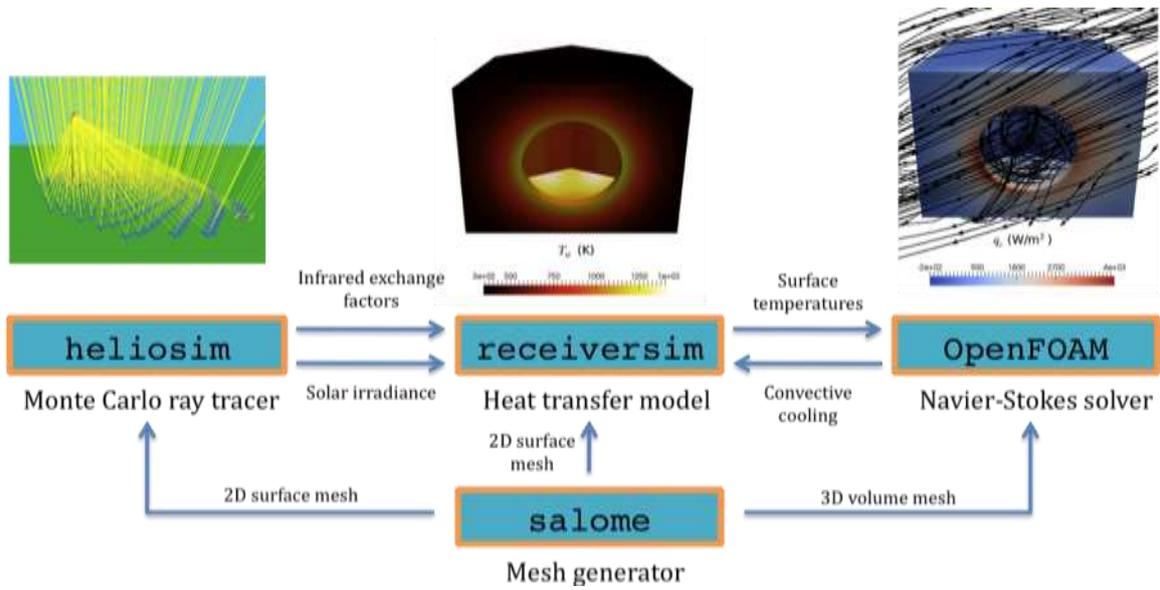
**Figure 2: Components of the integrated central receiver system model, and their interactions.**
