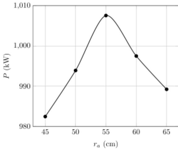
(a) Receiver thermal power output
