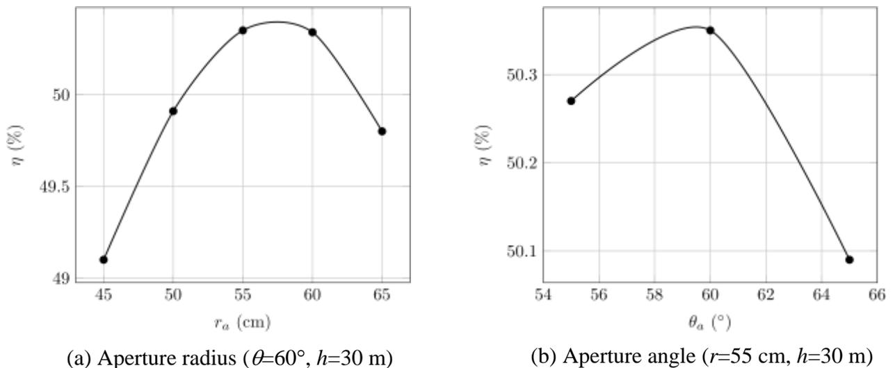
**Figure 6: Sensitivity of annual thermal efficiency to aperture and tower parameters.**
