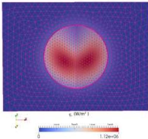
(a) Solar irradiance on all receiver parts with surface mesh shown.
