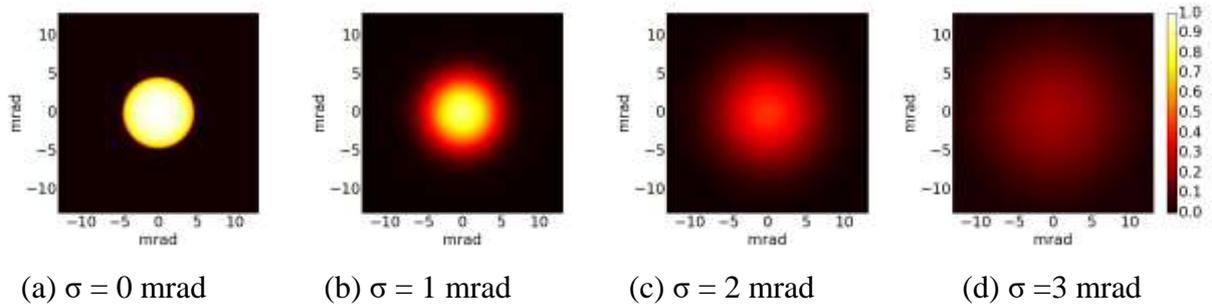
**Figure 4: Normalised solar irradiance of degraded sun shapes for a range of mirror slope and tracking errors ( $\sigma$ ).**
