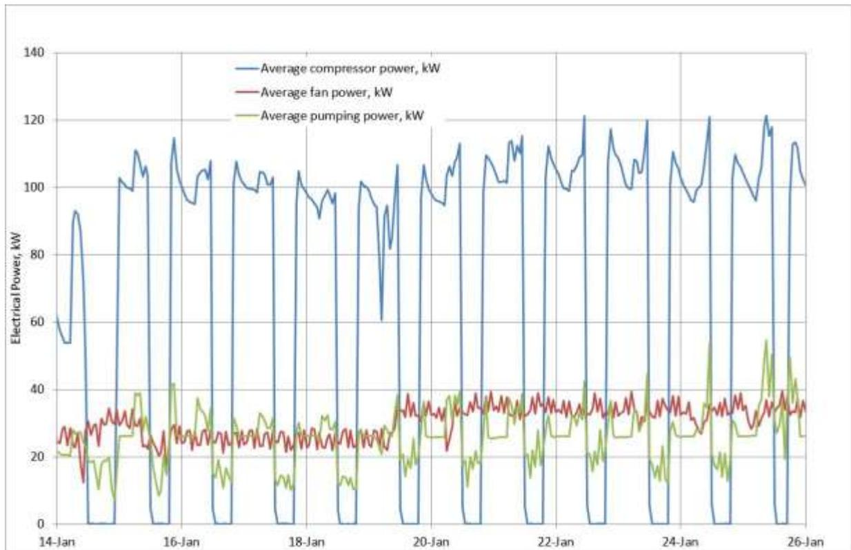
Figure 3. Electrical power profile of refrigeration system during operation in January 2015.
