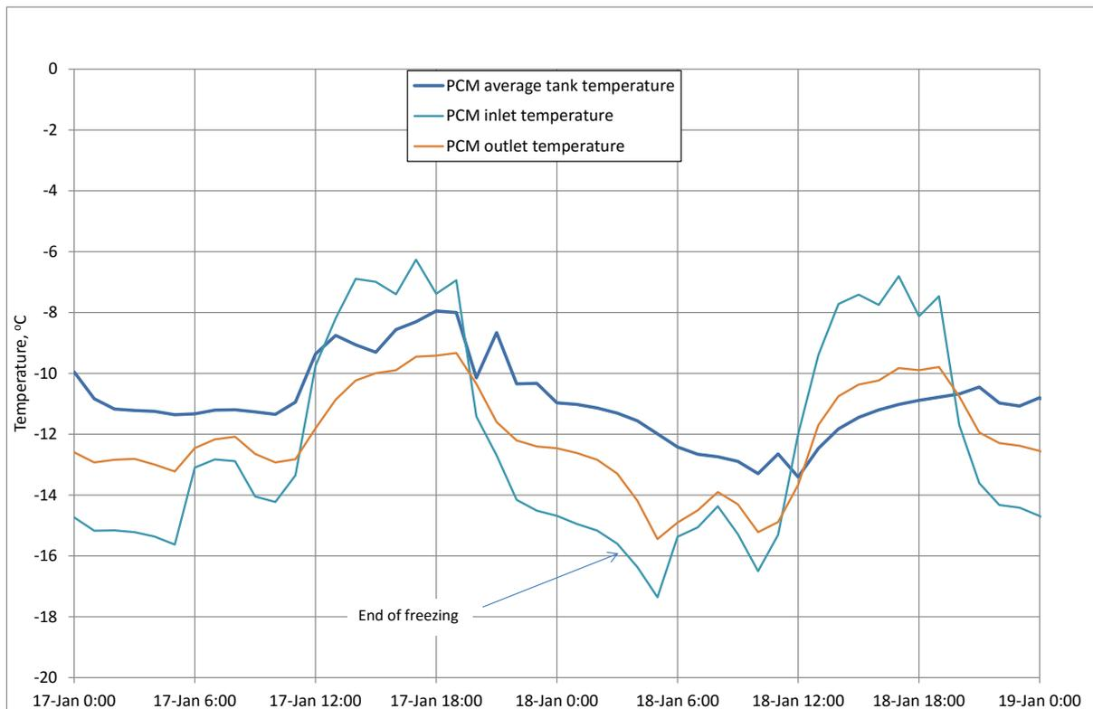
**Figure 5. Temperature profile during charging/discharging cycle 18 January 2015, showing complete charging.**
