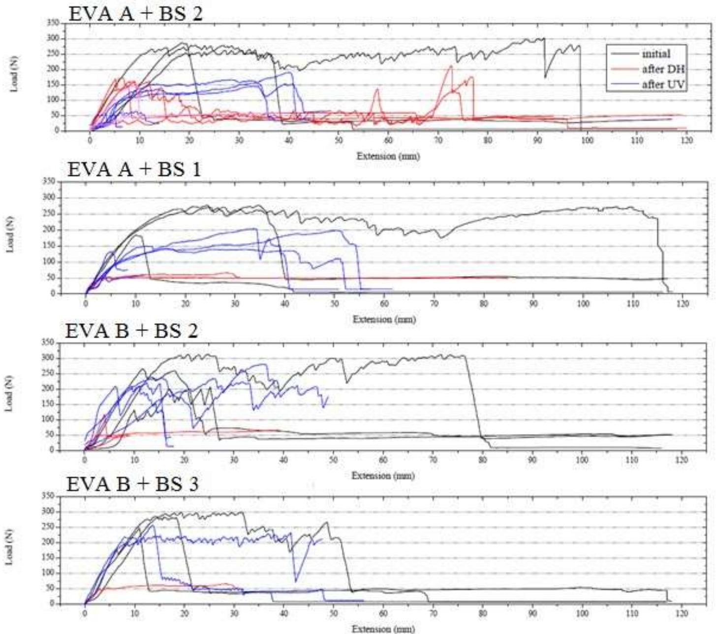
Figure 3: Peel tests for DH samples were exposed for 2600 hours and UV samples were exposed to 119 kWh/m<sup>2</sup> of UV (280 – 400nm). Loadings of ~50N experienced backsheet rupture and EVA stretching.
