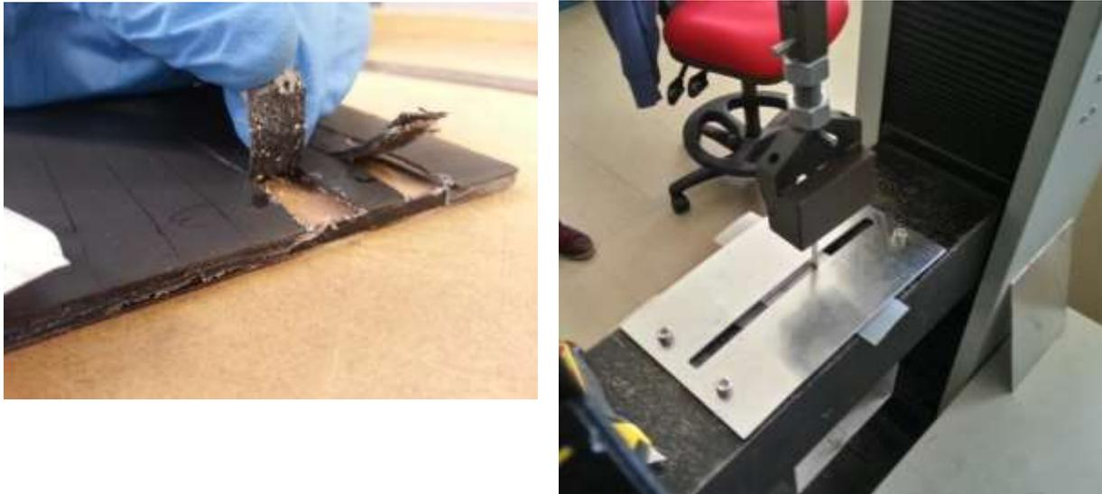
Figure 2: Sample made ready for the peel test (Left) and a sample held in the Instron during the peel test (Right)
