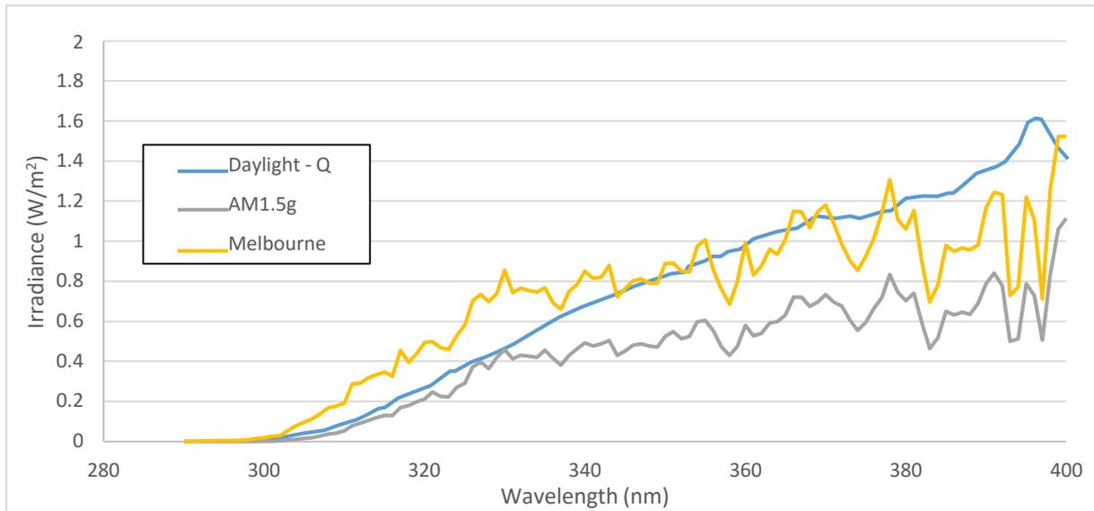
Figure 1: Comparison of UV spectrum for the Daylight - Q filter and modelled outdoor conditions
