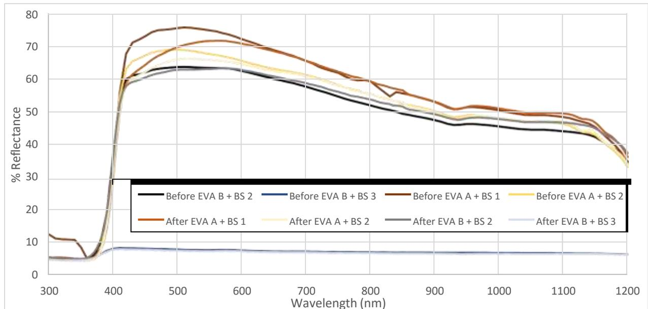
Figure 5: Spectrophotometry from 300-1200nm of DH samples after 2500hours of exposure
