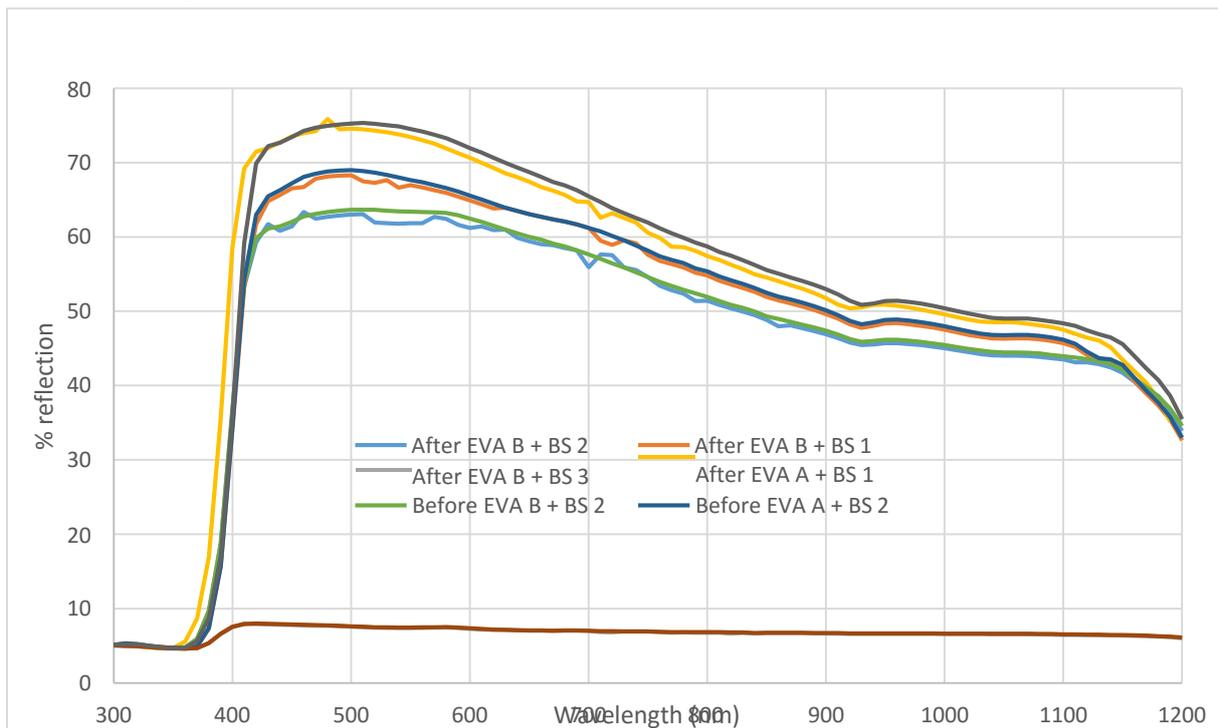
Figure 4: Spectrophotometry for UV degraded samples before and after 119 kWh/m<sup>2</sup> total UV dosage.
