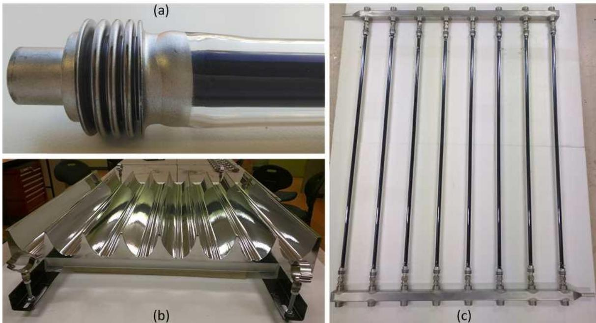
**Figure 7. Prototype Collector: (a) close up of evacuated tube bellows, (b) aluminium sputtered RenShape CPC, and (c) absorber tube and manifold assembly.**
