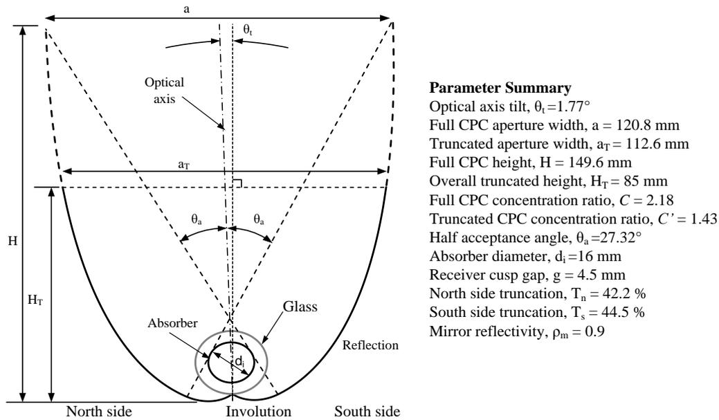
Figure 2. Geometry of symmetric CPC, rotated and asymmetrically truncated.
