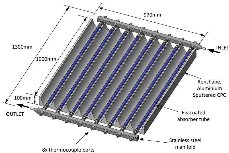
**Figure 6. CAD representation of the collector prototype being tested at RMIT.**
