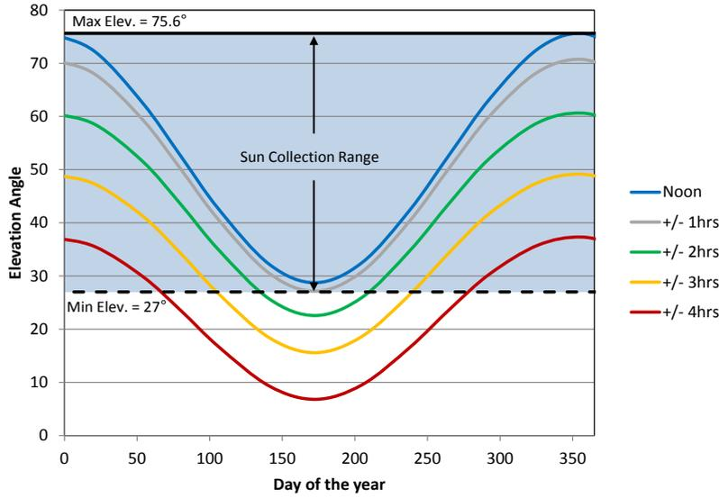
**Figure 1. Sun elevation angle for Melbourne showing the acceptance band for this CPC collector.**
