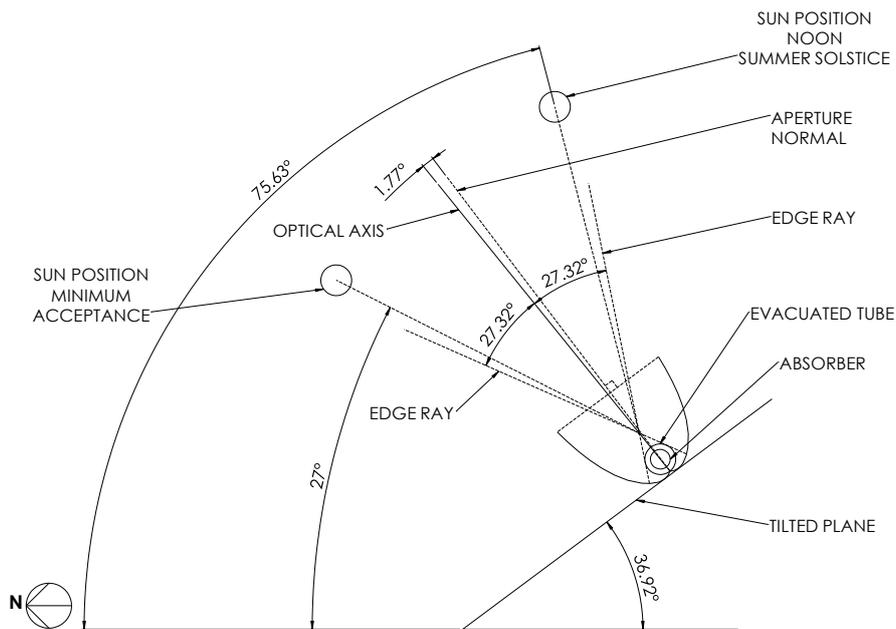
Figure 3. Geometry of symmetric CPC, asymmetrically truncated – View facing East.
