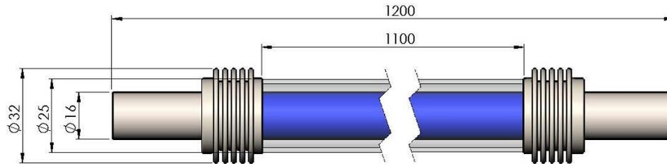
**Figure 4. Evacuated absorber tube dimensions**
