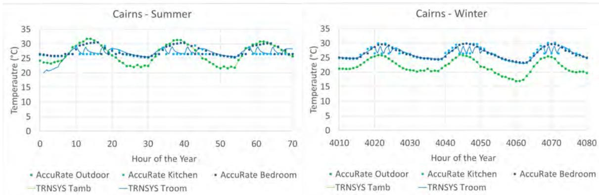
**Figure 3: Cairns Occupied Space Temperatures**
