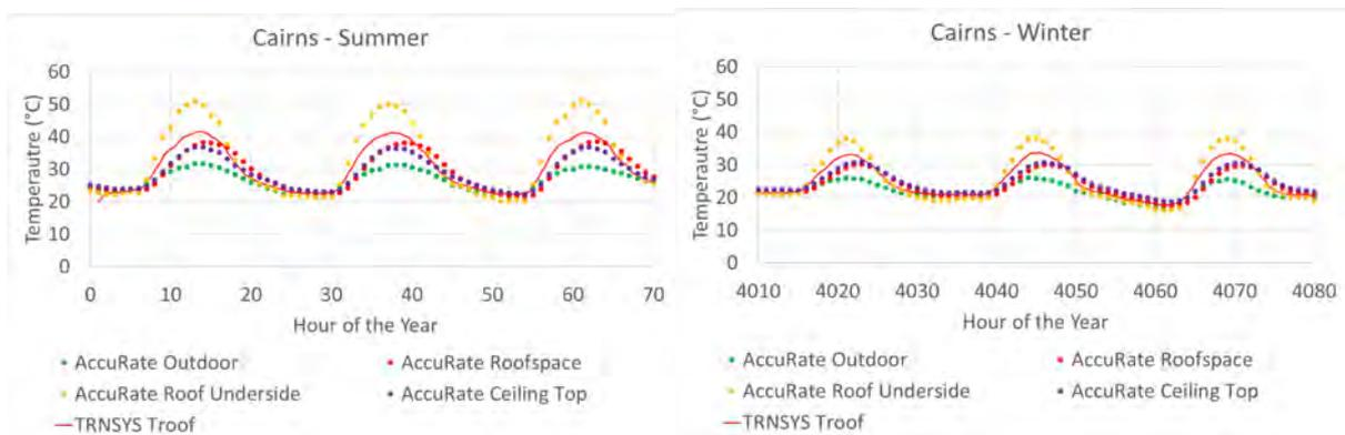
**Figure 5: Cairns Roof Space Temperatures**
