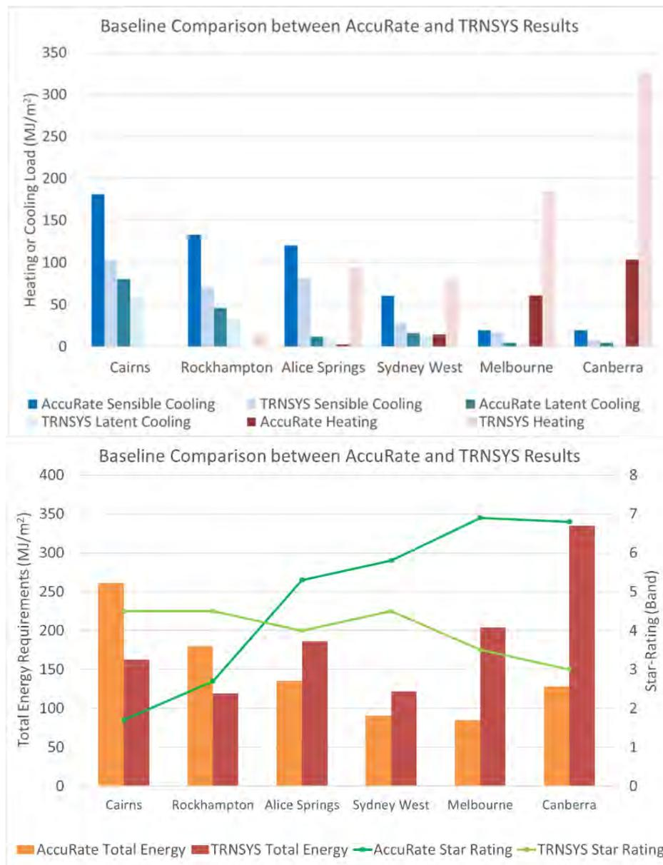
**Figure 1: Baseline Comparison between TRNSYS and AccuRate Results**
